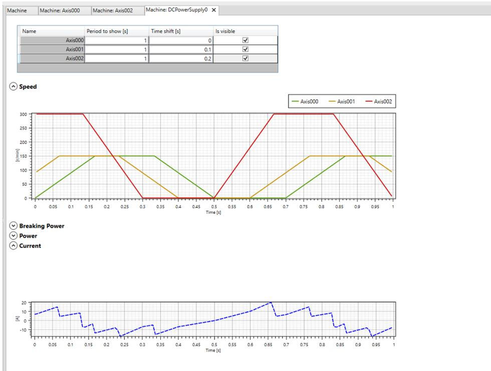
You can add an axis time shift to align the different axis profile to the real machine operation. Those profiles will be summed to obtain the profiles for Braking power, total power and current needed.
