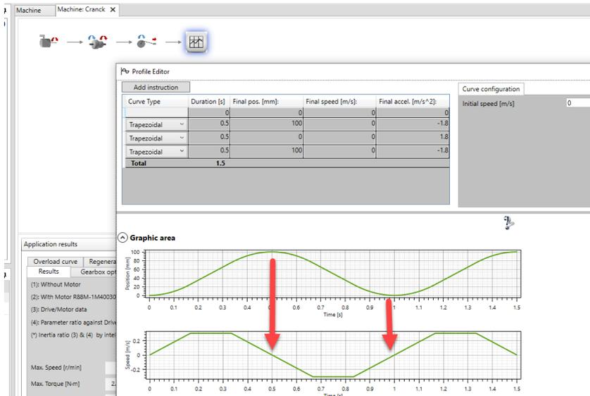
In addition, if the commanded position is out of range it is indicated with a warning.
