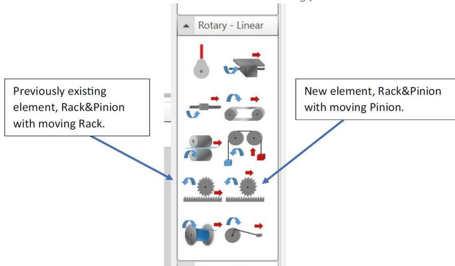
In this element, the motor moves the pinion (directly or via other rotary element) and the pinion and all the elements from pinion to the motor moves linearly.
