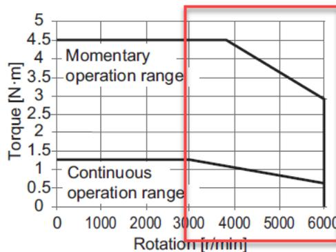
If the application requires that the motor moves in the speed range above rated speed, we have to consider this torque derating at the actual instantaneous speed.
