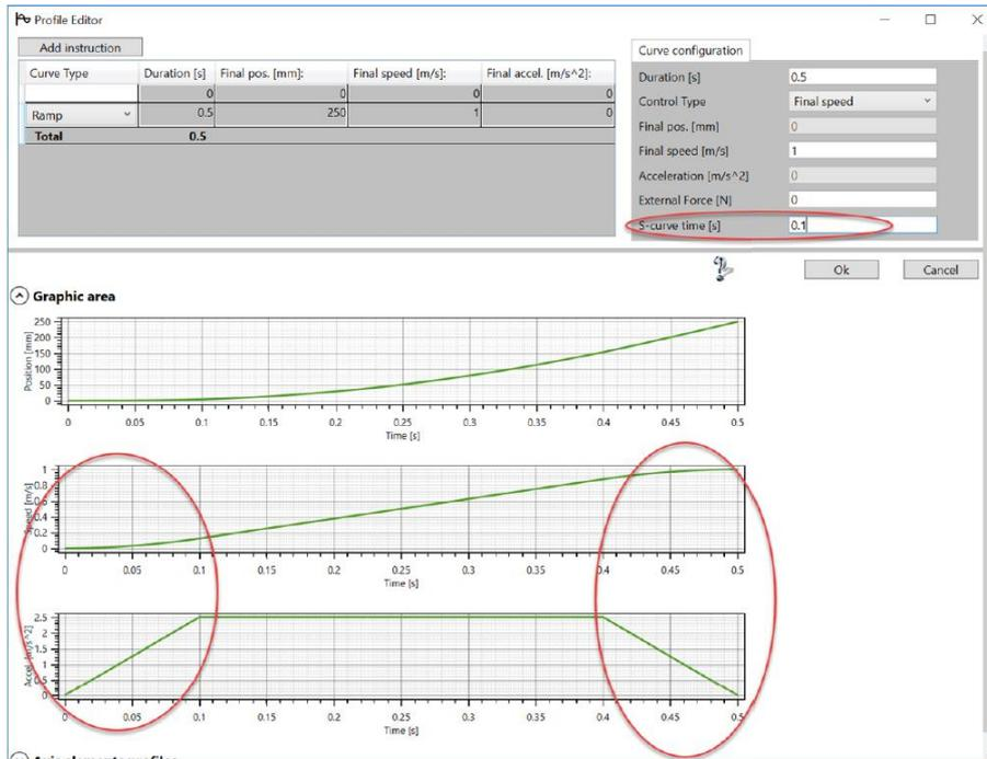
The S-curve time is added at the start and at the end of the Ramp segment. Obviously, the time range is from 0 (default) to "Duration/2" (all ramp segment is S-curve).
