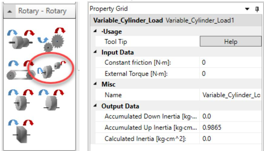
When this element is included in a kinematic chain we impose the restriction that this should be the last mechanical element, just before the profile:
