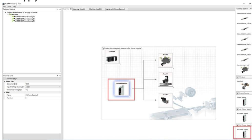
Supplying the servodrives via DC bus is becoming more and more common because this allows to reduce the use of energy by sharing the DC-bus of several drives. Then, when one servomotor is regenerating energy when decelerating or holding a vertical load, this energy can be used by another motor that is motoring.
