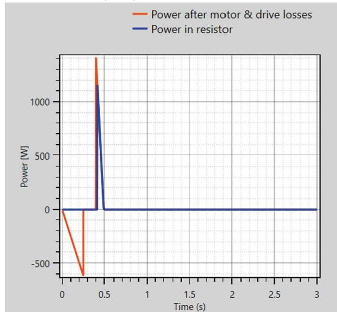
In previous versions, the Regeneration power was calculated only based in the total-cycle averaged regenerative power. This results in abnormally small power resistors in applications with very long dwell time. In Version 1.5 we have set a limit in the ratio between regeneration power during deceleration and regeneration power in all the cycle.
