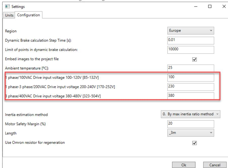
You can link to the AC power supply any drive with the same voltage range.
