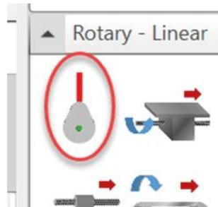
This kind of mechanical elements are designed to run the motor at constant speed and the CAM lifts up & down some kind of mass. For this reason, the motion profile should be in motor side.
