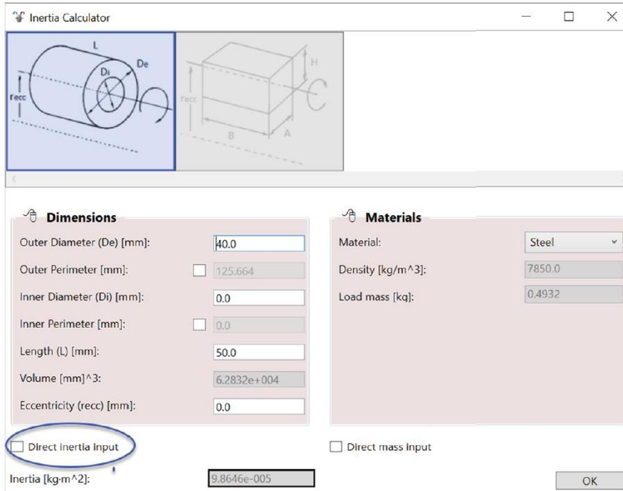
The gearbox keeps by default Direct inertia Input as Inertia is a data that is normally given by the gearbox maker.
