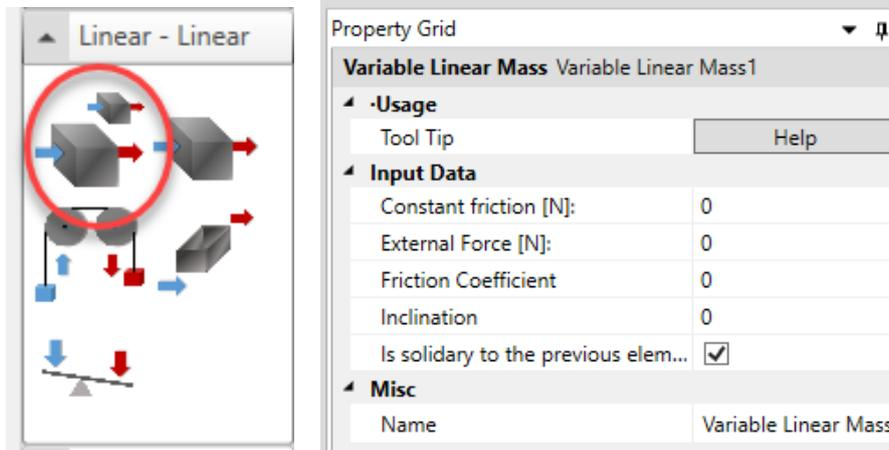
When this element is included in a kinematic chain we impose the restriction that this should be the last mechanical element, just before the profile:
