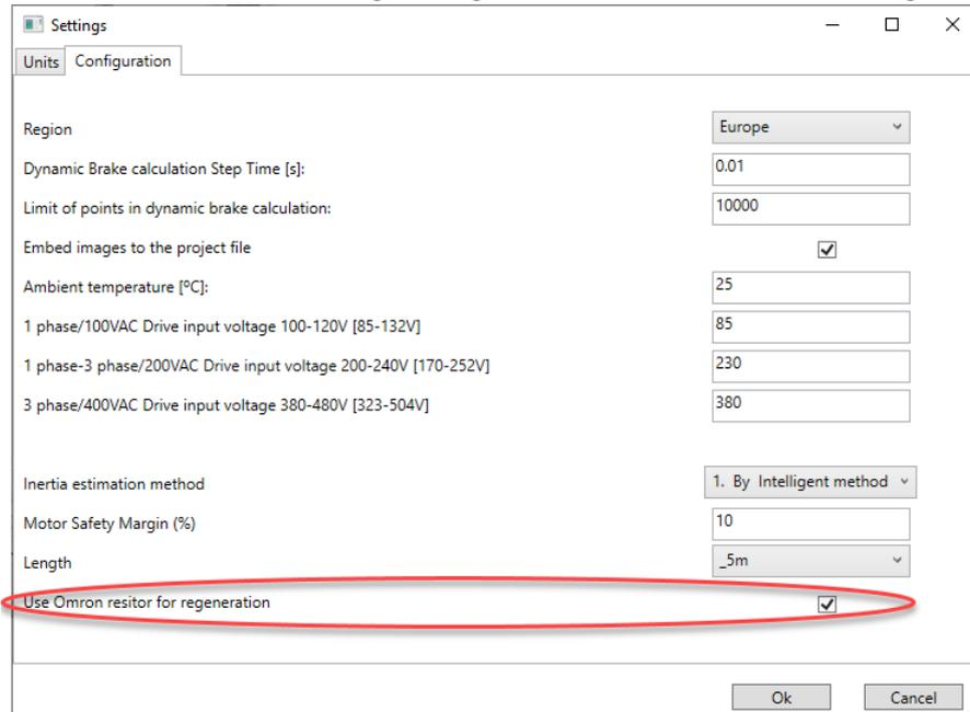
In addition, if the Maximum Torque of the selected motor is exceeded the braking resistor is not calculated because the result is unrealistic.
