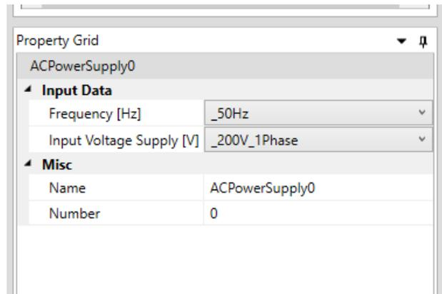
Frequency can be 50Hz or 60Hz
