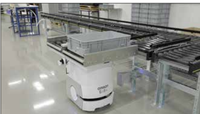
Omron LD robots have replaced roller conveyors, leading to a more flexible production and logistics set-up.
