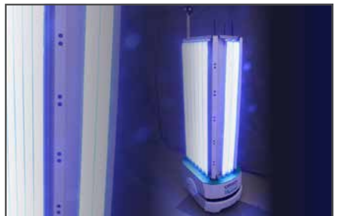
Comprising an array of precision UV-C lamps developed by Phillips and mounted on top of an OMRON mobile robot platform, the UV-C Robot autonomously navigates the natural features of a facility,
