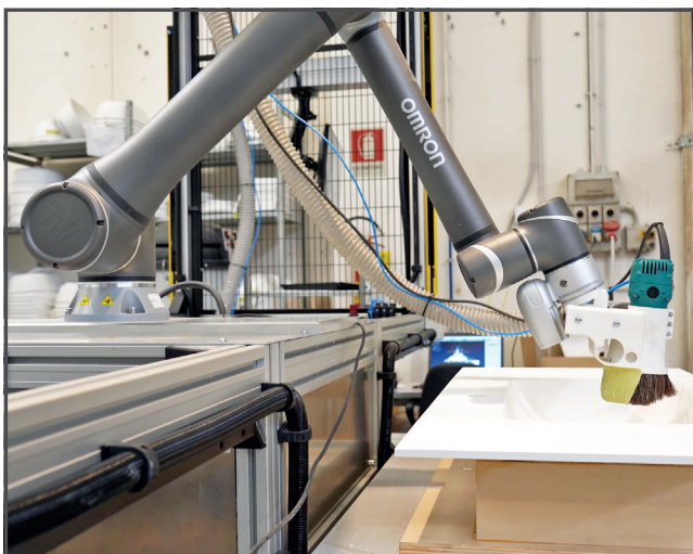
The cobot is used to automate all the finishing operations of Topcustom's products made from Ocritech.
