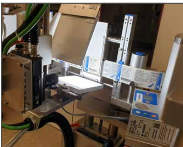
With the help of the FHV7 inspection system, the HERMA labelling machine at Steierl-Pharma checks the identity of the label based on the pharmaceutical code and verifies batch and expiration.
