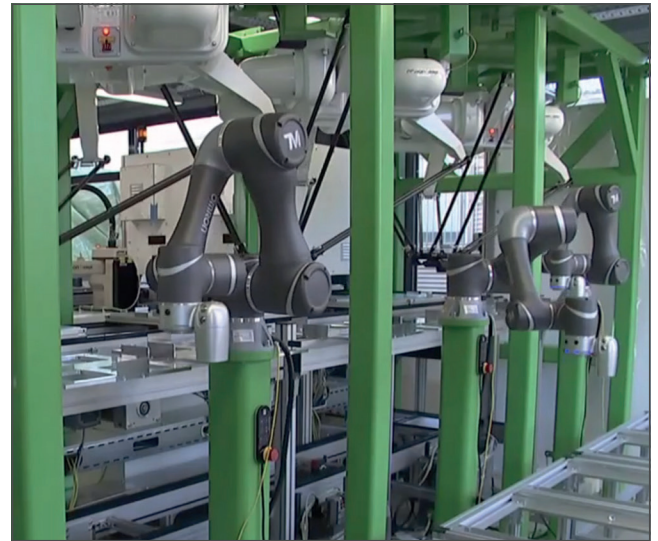
The cobot relieves employees of recurring tasks involving test cutting and packaging and helps to increase productivity.
