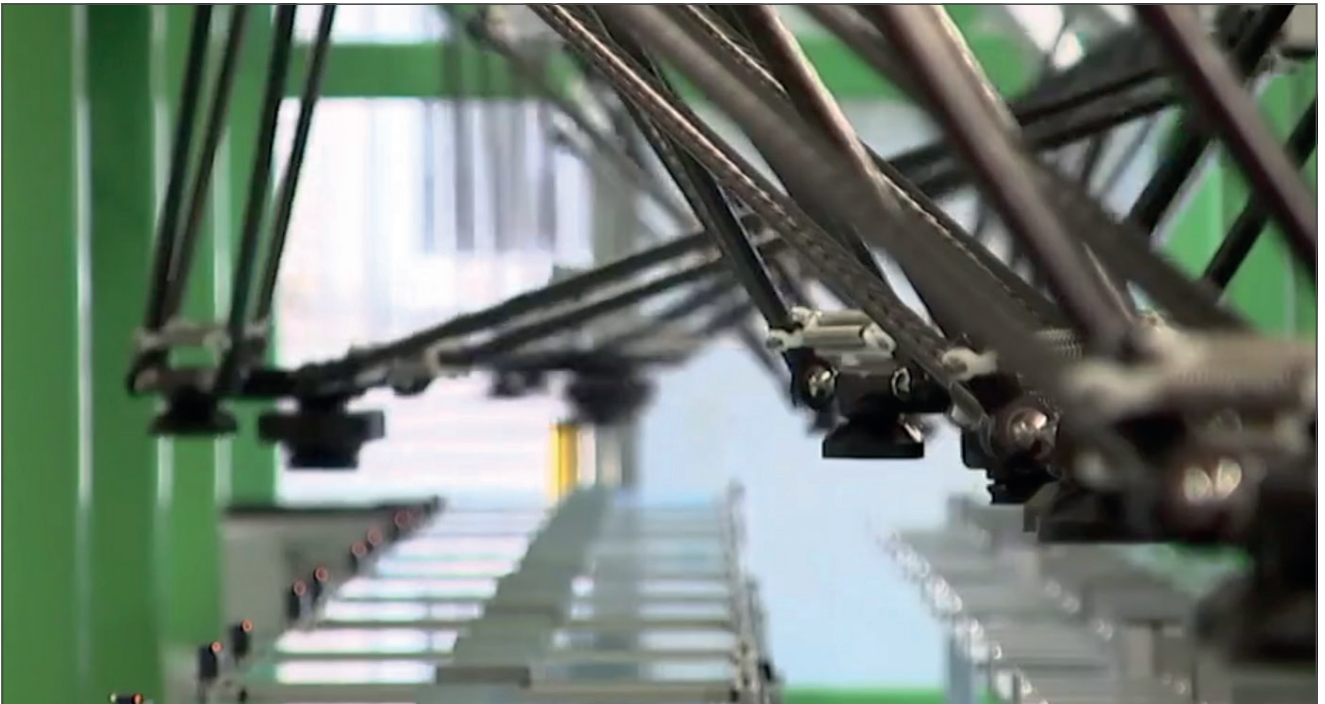
Components of the flexible COVID-19 test kit production include the Quattro 650 H four-axis parallel robots.
