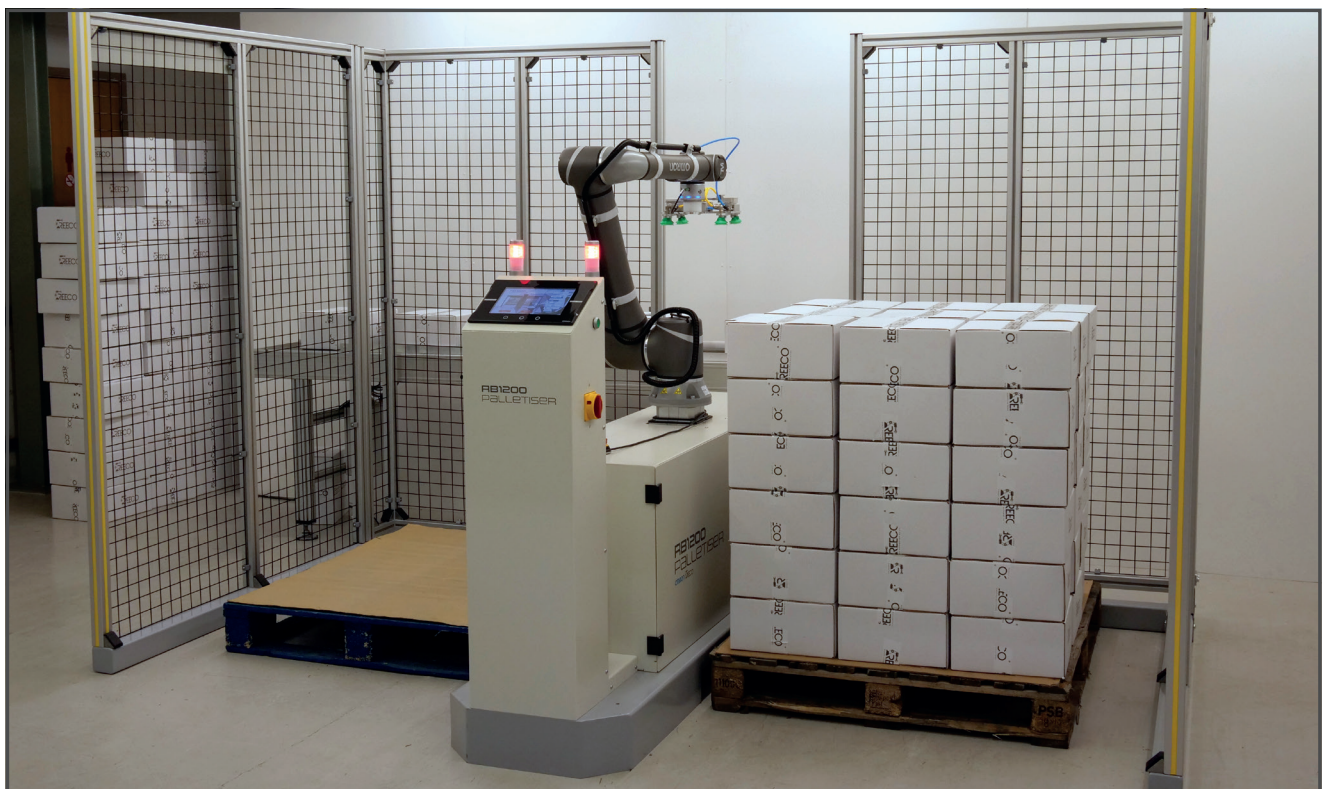
Measuring just 2.2 x 3.2m, the RB1200's footprint is 60% smaller than a typical 4x4m cartesian palletiser
