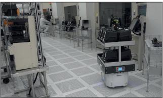
The implementation of the solution involved deploying a fleet of seven robots that efficiently transported materials from the main work-in-progress (WIP) storage area to various points within fabrication. OMRON's robots autonomously handle the transportation of materials over long distances, significantly reducing the need for manual intervention and improving overall efficiency in Polar's manufacturing process.
