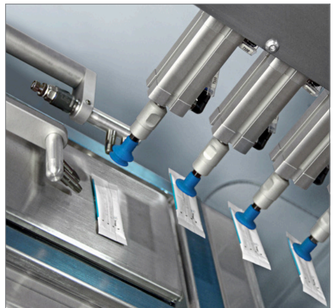
Automatic system for the statistical control of weight online
