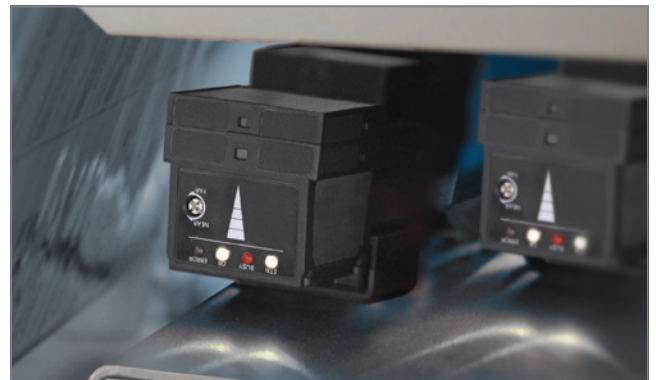
Each camera Smart Camera FQ2 reads what he has written the laser marker and sends it as a string to the PLC via Ethernet to be compared with the data information entered by the operator. The presence of a film of wrapping material has polished led to the use of a system of lighting anti-glare.
