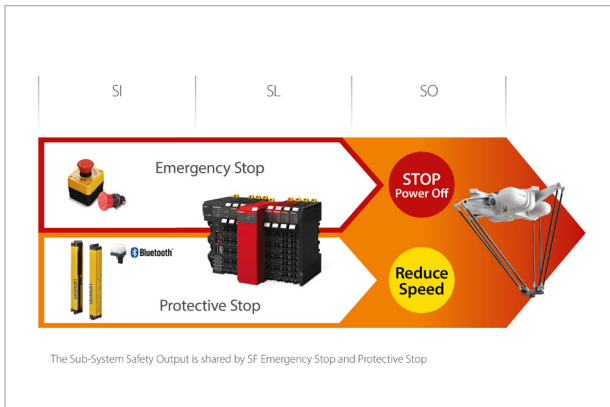
The sub-system safety output is shared by SF Emergency Stop and Protective Stop.
