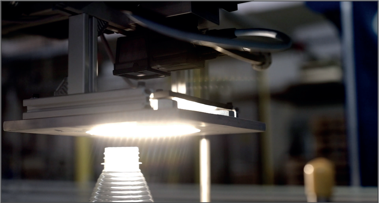
The OMRON system is used on the production line, and incorporates lights and cameras set at different angles so that they can detect any defects.
