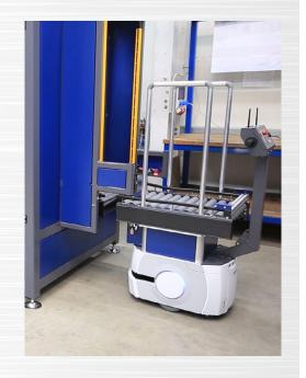
The Precision Drive function allows the robot to position itself very accurately in front of the conveyor belt. Additionally, it supports gentle start-up and braking processes, which is crucial when transporting fragile and expensive materials.
