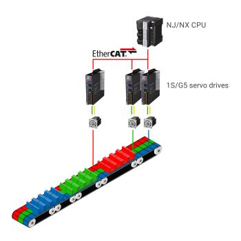
Very fast and accurate processes required the use of 15 OMRON 1S servo drives with a cycle time of 0.5ms, which enabled the packaging processes to be completed. The entire machine was programmed using ready-made function blocks for drive synchronization, based on several CAMs, which are predefined computer aided motion profiles for the actuating drives. The built-in graphical CAM editor enabled intuitive preparation of the appropriate drive motion profiles.
