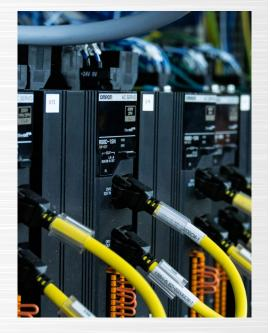
Very fast and accurate processes required the use of 15 OMRON 1S servo drives with a cycle time of 0.5ms, which enabled the packaging processes to be completed.
