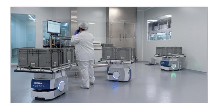
warehouse. This includes the transportation of 700 boxes of vials each day, with each load weighing 70kg. Associated with this was the need to feed empty boxes into the system and to manage the opening of doors whilst maintaining a 100% clean environment.
