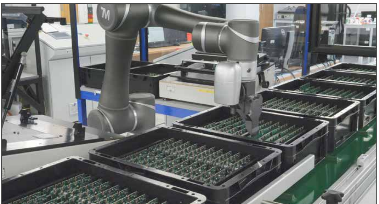
The cobots have special tooling that allow them to open and shut the manual testing equipment.
