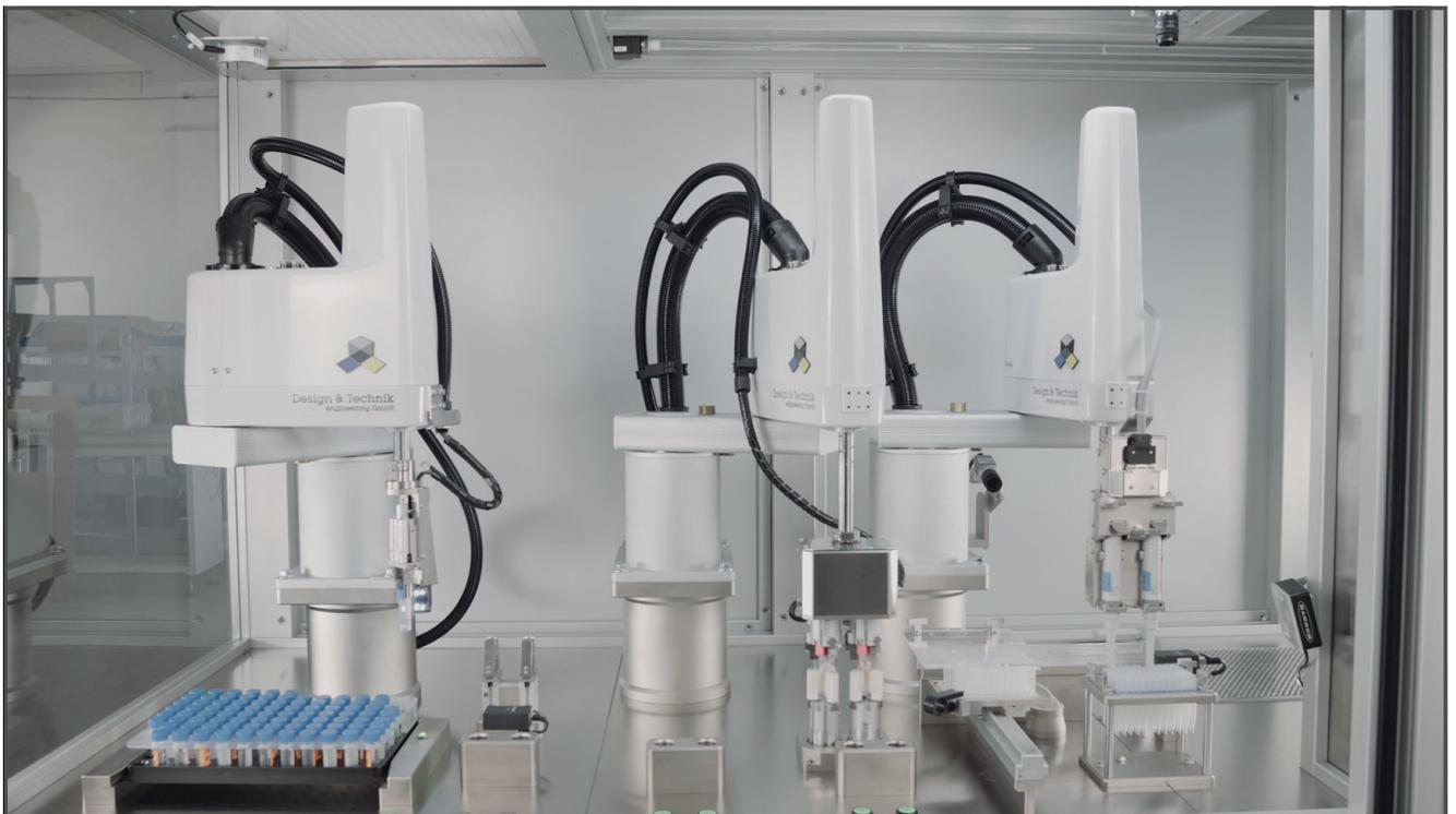
*The PT600 laboratory processing system uses an OMRON Cobra 450 robot for contactless transport.*
