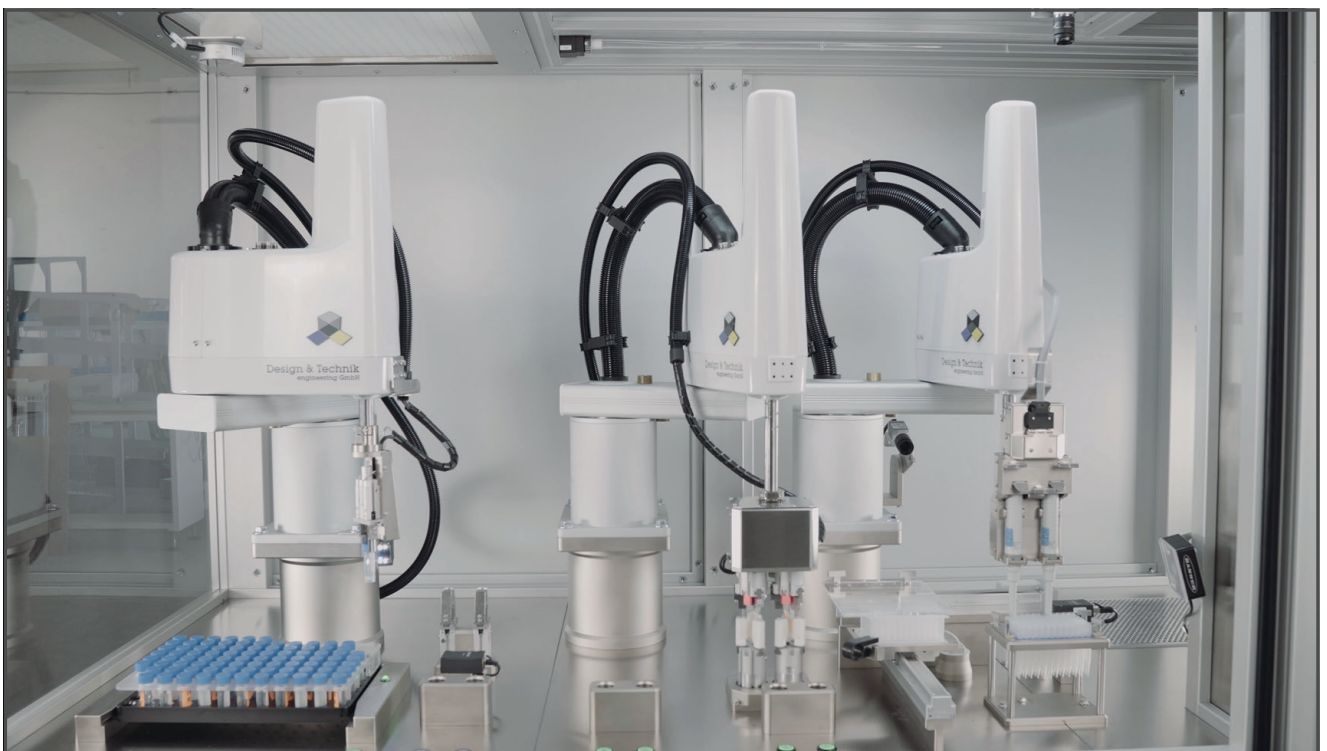
The PT600 laboratory processing system uses an OMRON Cobra 450 robot for contactless transport.
