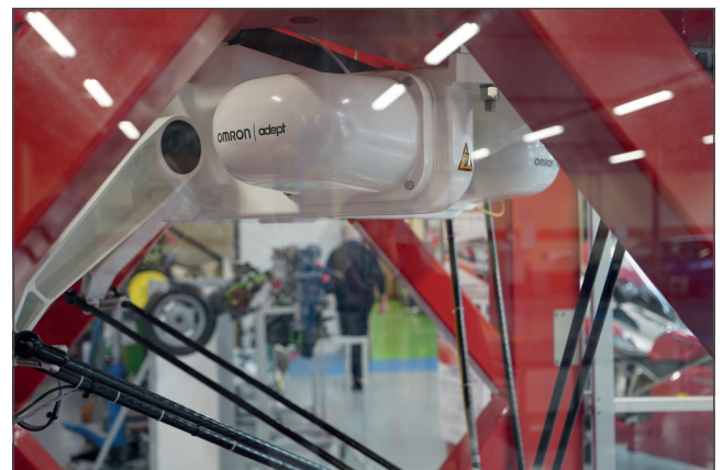
The solution can replicate, on three axes, the effect of speed, acceleration and deceleration on the movement of a black box installed in a car.
