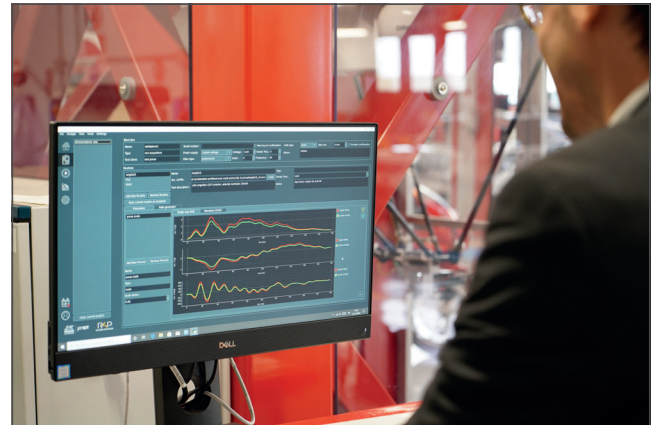
The solution uses Omron's Delta Quattro robot, which is programmed to subject the black boxes to the same acceleration and deceleration that would be recorded on a car during a crash test.
