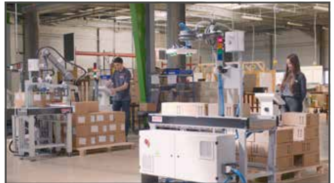
The palletising solution allows collaboration with operators, who can work in safe proximity to the cobot without fencing.
