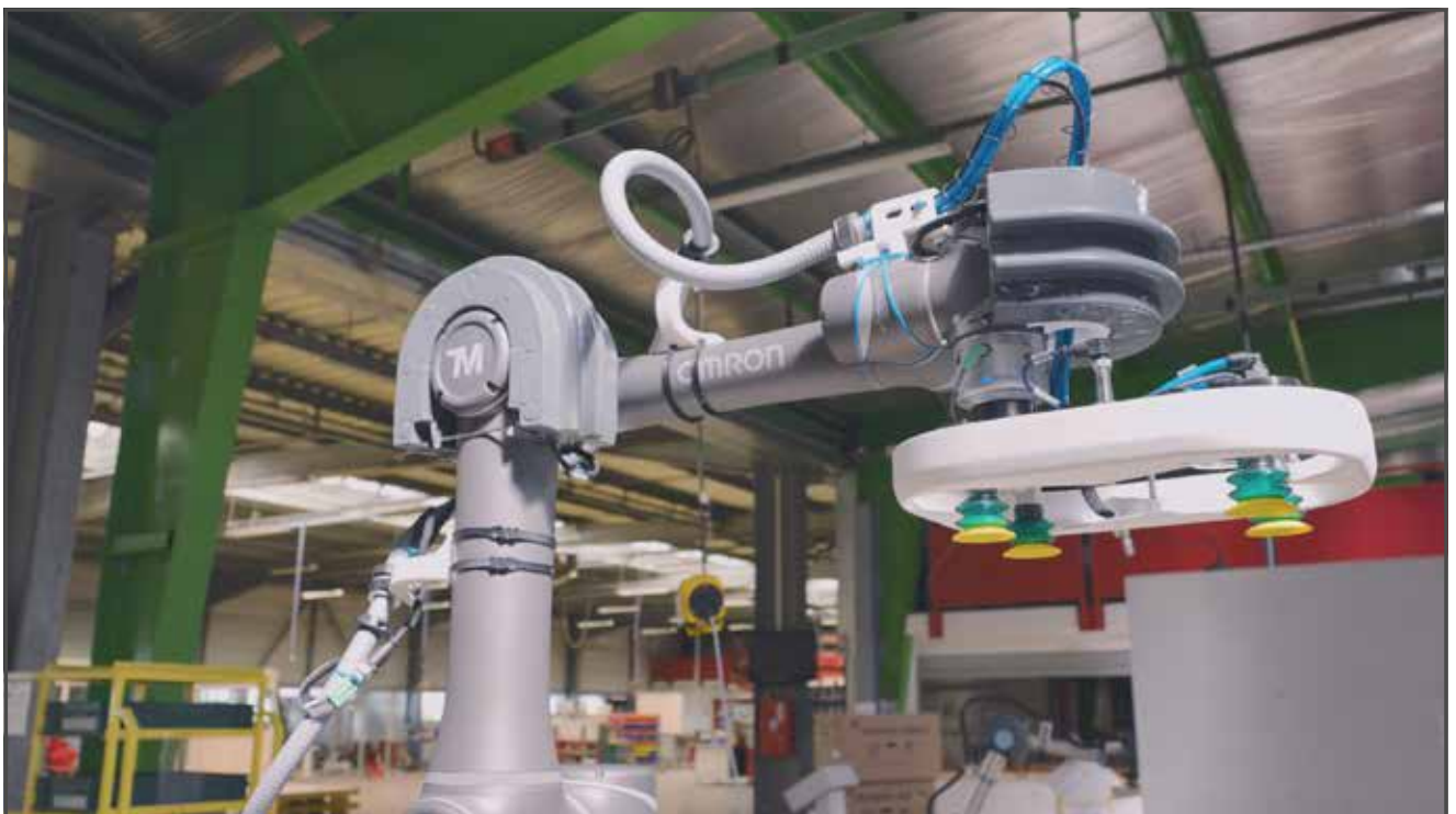
Cobot palletising solution with small footprint and active safety equipment enables handling up to 8 boxes per minute.
