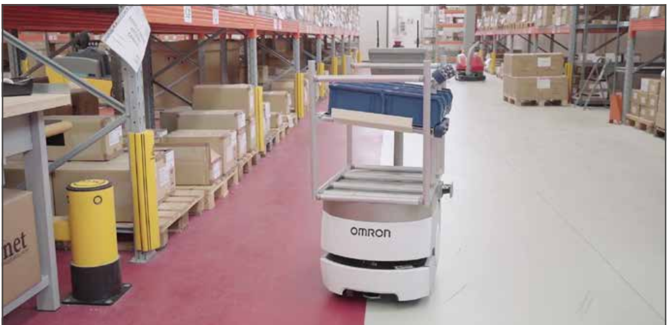
FasThink designed and developed a material handling solution with its proprietary Pick-to-Light (P2Light) technology and OMRON's mobile robots.
