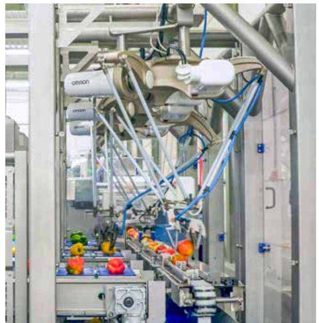
"We used three Omron robots in a waterproof variant that can be cleaned thoroughly."
