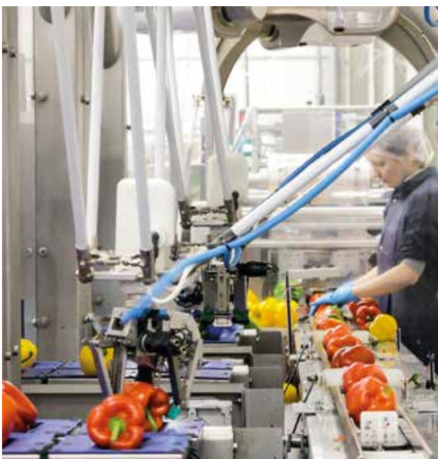
The robots pick up the bell peppers and correctly position them on the belt in the correct colour order.
