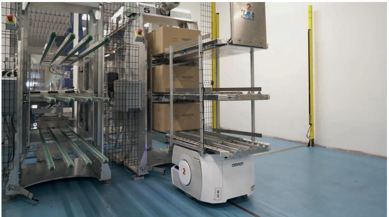
The AMRs can move independently within the work environment, deciding which path to take to the destination.
