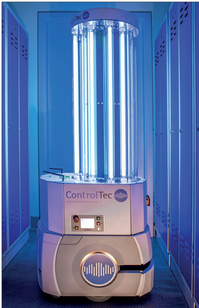
ControlTec devised the concept of the UVC robot to help fight against the virus.
