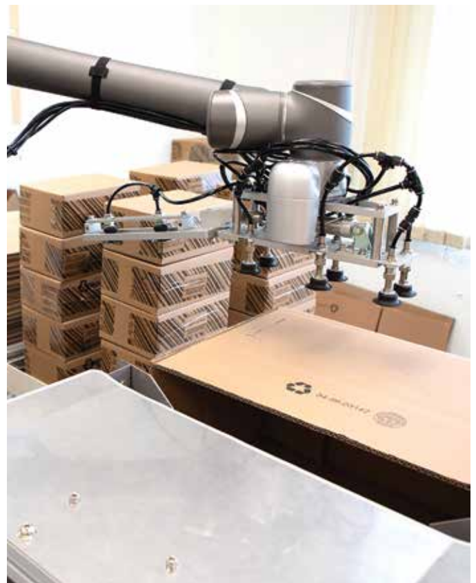
In a collaborative application, risk assessments must take into account any surrounding equipment in addition to the robot itself.
