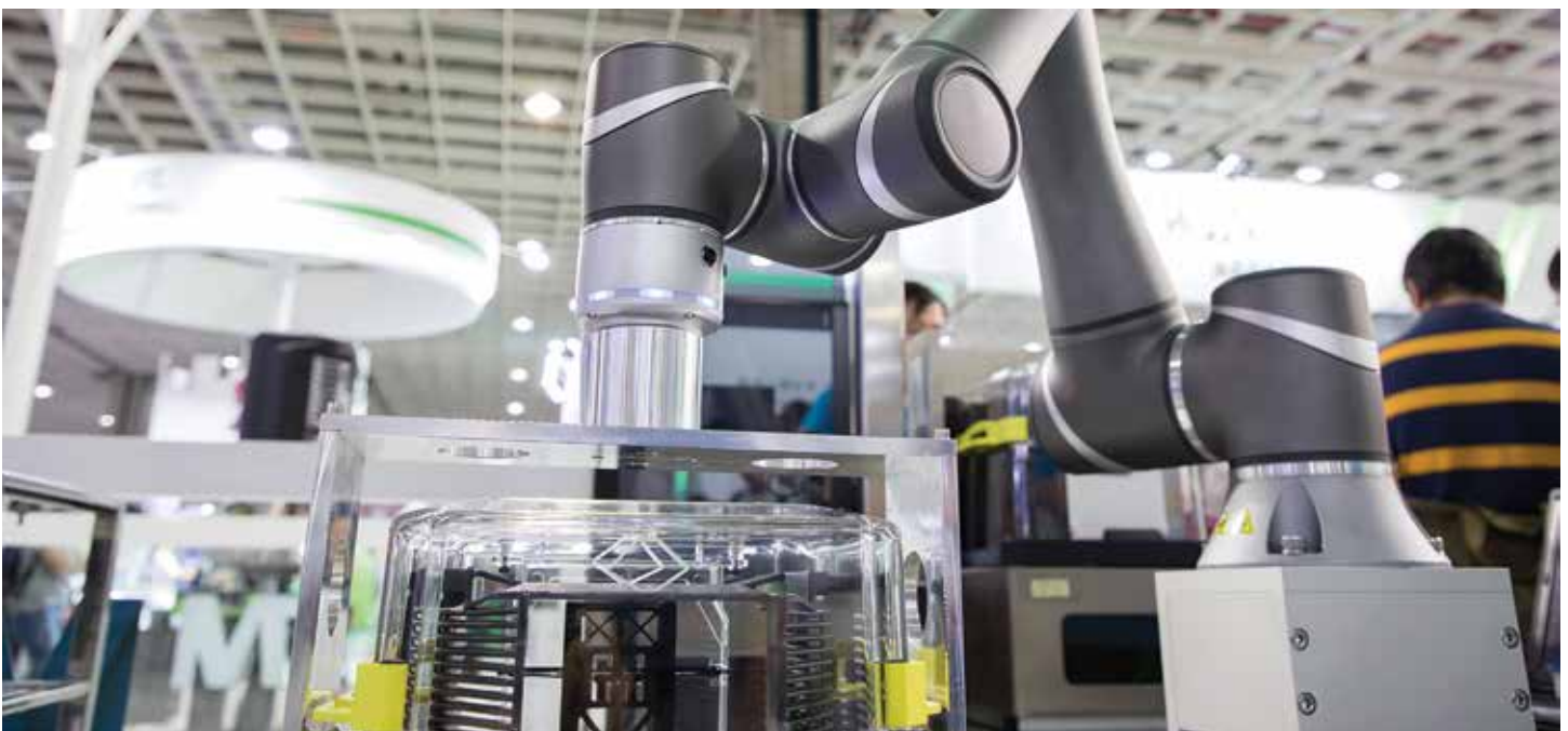
Collaborative robots generally support lighter payloads than standalone robots, but they offer greater flexibility.
