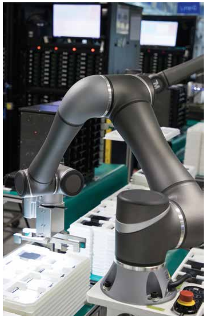
A collaborative robot's arm is lightweight and flexible, with minimal pinch points to ensure safe operation.
