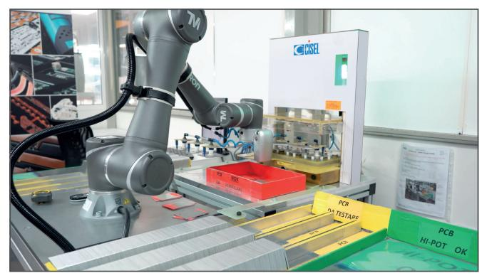
Cisel uses the OMRON TM5 cobot to automate the electrical testing of boards used in the power steering system of a leading automotive manufacturer.
