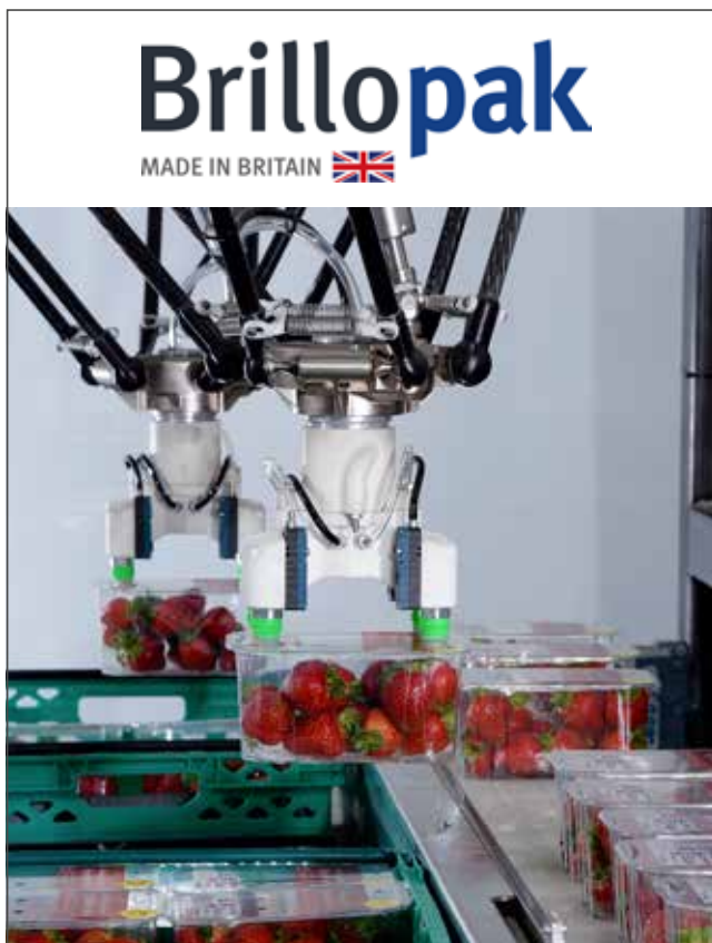
Brillopak developed a unique "single-pick" concept that loads each punnet to the correct place in the box with the help of the four arm Delta robot from Omron.
