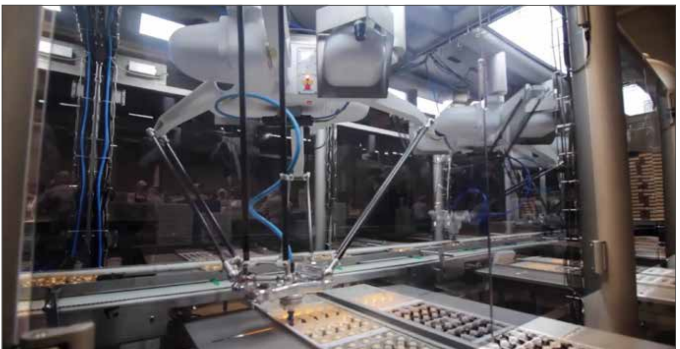
The three robots work in sync with each other as part of an integrated system that includes visual inspection, safety and the robotic systems.
