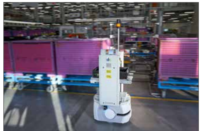
The autonomous mobile robots are equipped with a conveyor tower - a height-adjustable load handling device, developed by system integrator cts GmbH.
