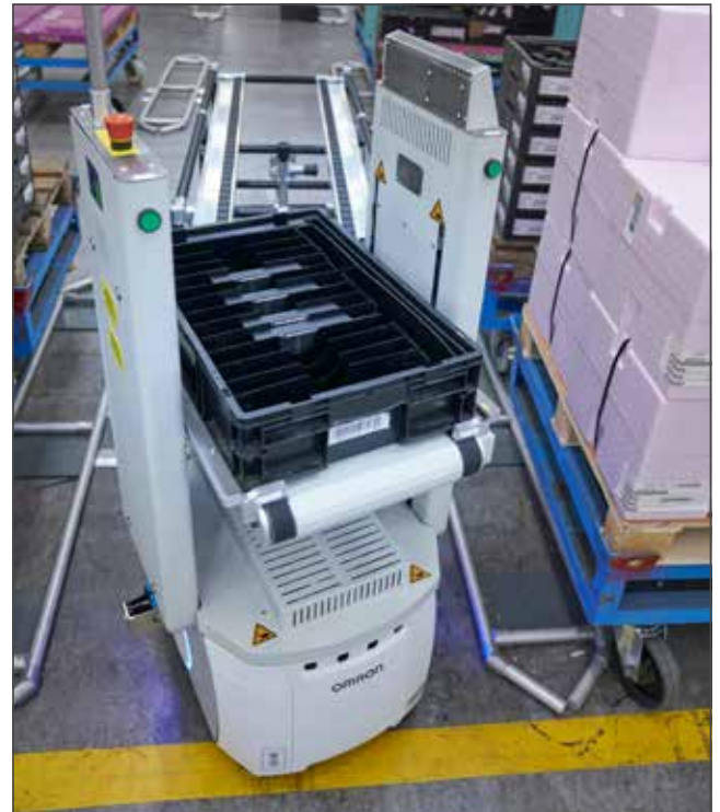
The delivery of urgent small parts is handled by the miniSTR based on the Omron LD mobile robot.
