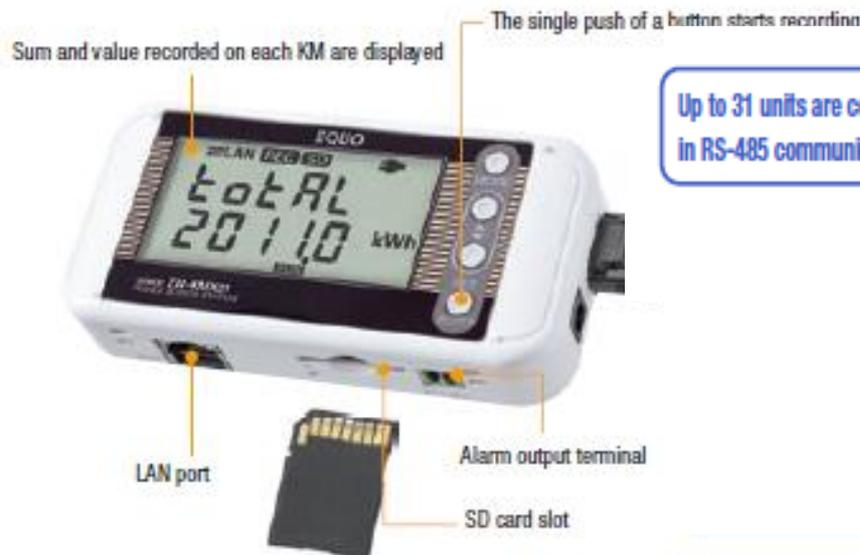
Up to 31 units are connectable in RS-485 communication
