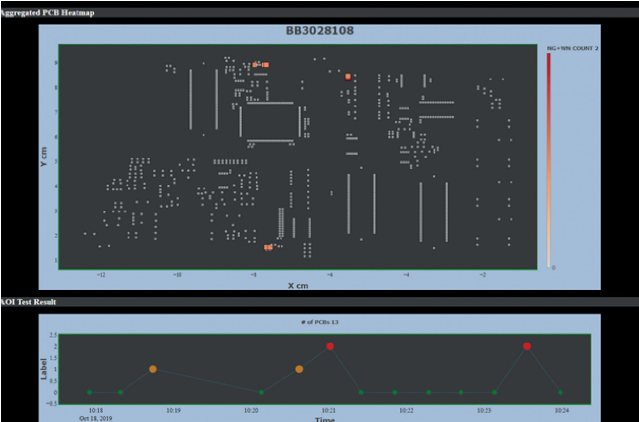
Fig. 5 – Operator dashboard showing solder application quality.
