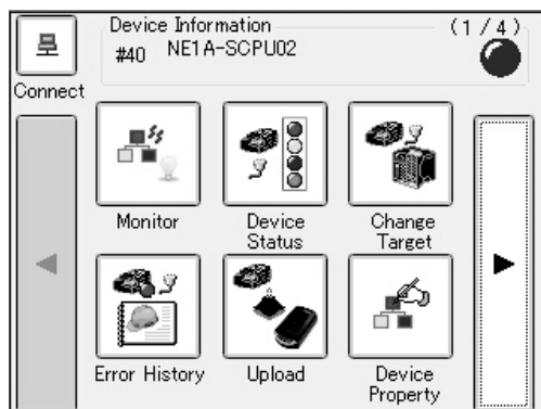
Main Window When Connected Online to a DeviceNet Safety Device
