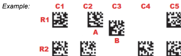
Symbol B is part of R1 if Minimum Same-Row Symbol Overlap Height Percentage is set to 20.
