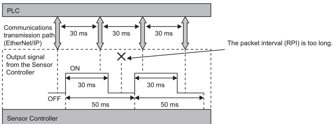
The PLC cannot detect some of the output signals from the Sensor Controller.
