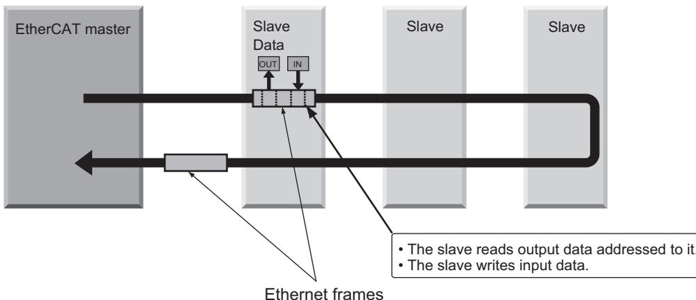
The data exchanges that are cyclically performed between the EtherCAT master and EtherCAT slaves use EtherCAT telegrams that are stored directly in the Ethernet frames. Each EtherCAT telegram consists of a telegram header (including the data length and one or more slave addresses), data, and a working counter (i.e., check bits).
