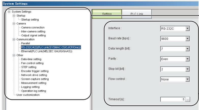
1. On the Main Window, select [Tool] – [System Settings]. Select [System data] from the tree on the left, and then select [Communication] – [RS-232C/422 (PLC Link (SYSMAC CS/CJ/CP/One))].
