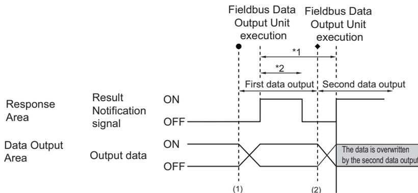
\*1, \*2: Data is output at the set output period\*<sup>1</sup> and for the set output time.\*<sup>2</sup> After data is output, the Result Notification signal is turned ON and the data is held for the data output time.
