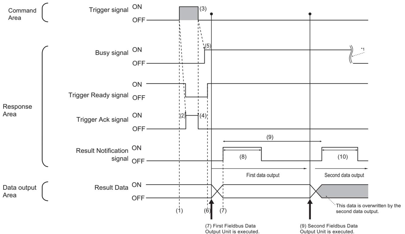
\*1: Busy (BUSY) signal is automatically switched ON from OFF when the command execution is completed.
