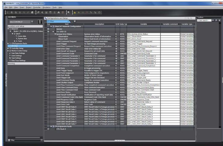
Right-click a slave or I/O port in the I/O map and select [Create Device Variable]. The device variable name is automatically created as a combination of the device name and the I/O port name. You can also select an I/O port and enter a variable name in the [Variable] column.
