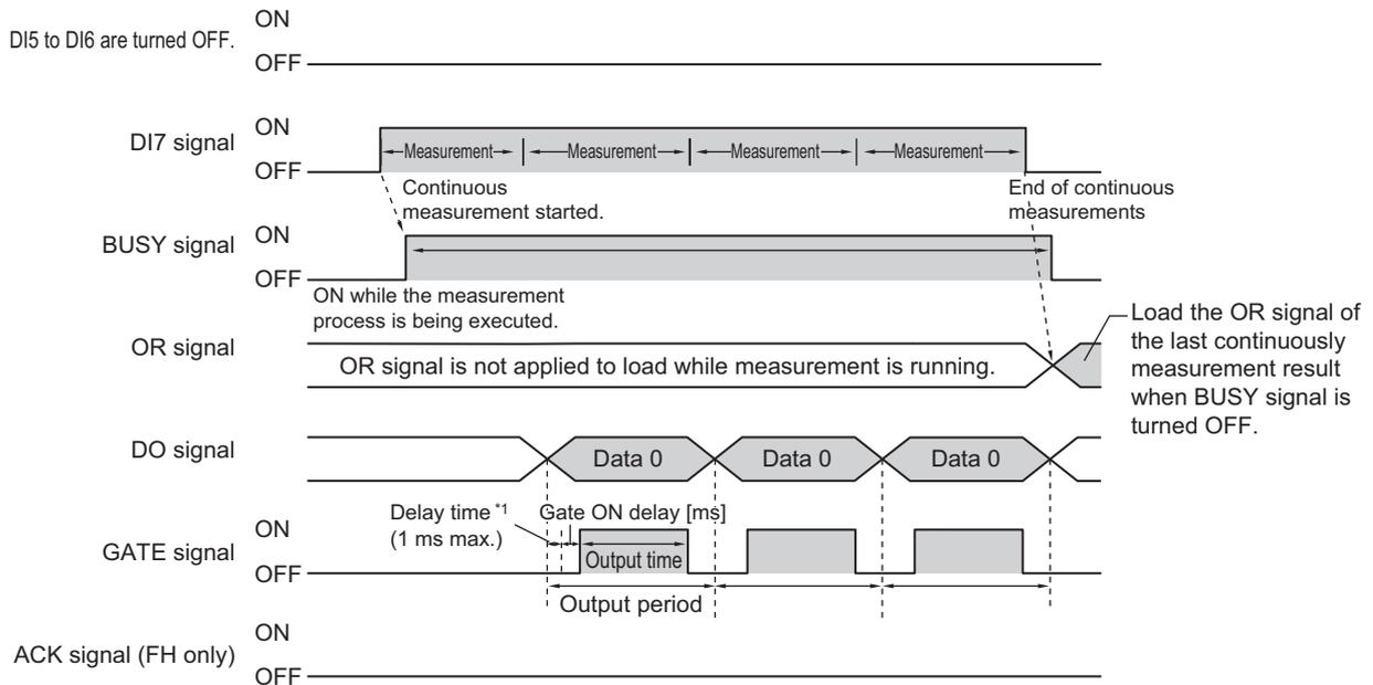
\*1 A delay of up to 1 ms will occur when the GATE signal is turned ON. (This applied only to the FH.)
