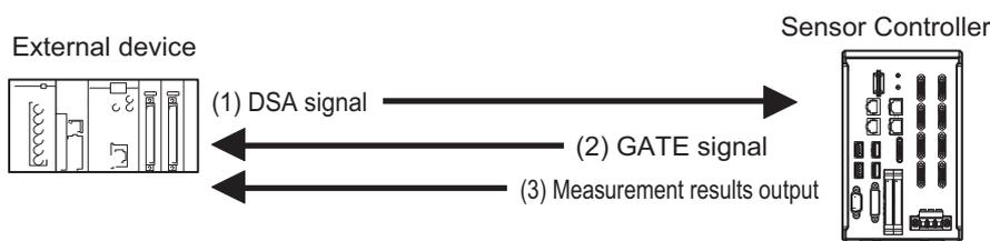
(1) The PLC turns ON the DSA signal and waits for the output data.
