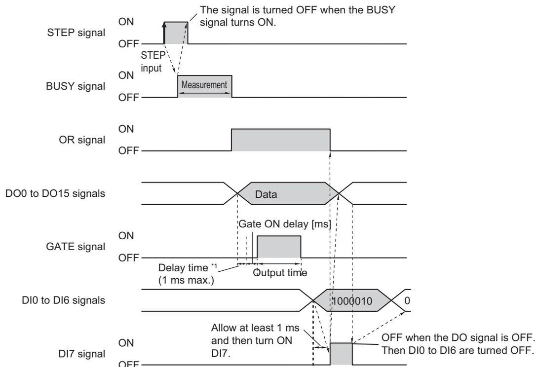
\*1 A delay of up to 1 ms will occur when the GATE signal is turned ON. (This applied only to the FH.)
