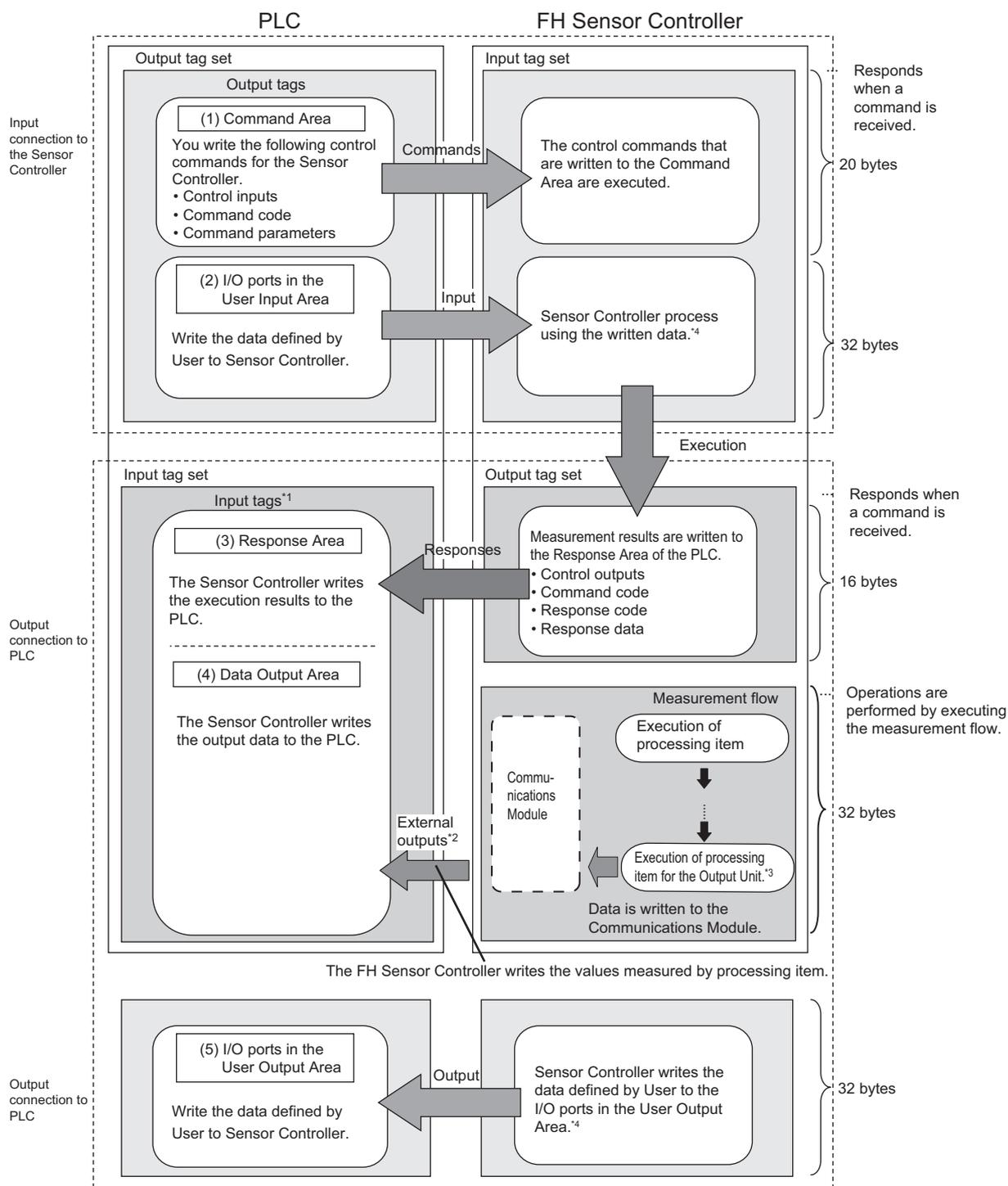
\*1: The Response Area (3) and Data Output Area (4) are assigned to continuous memory addresses or to variables.
