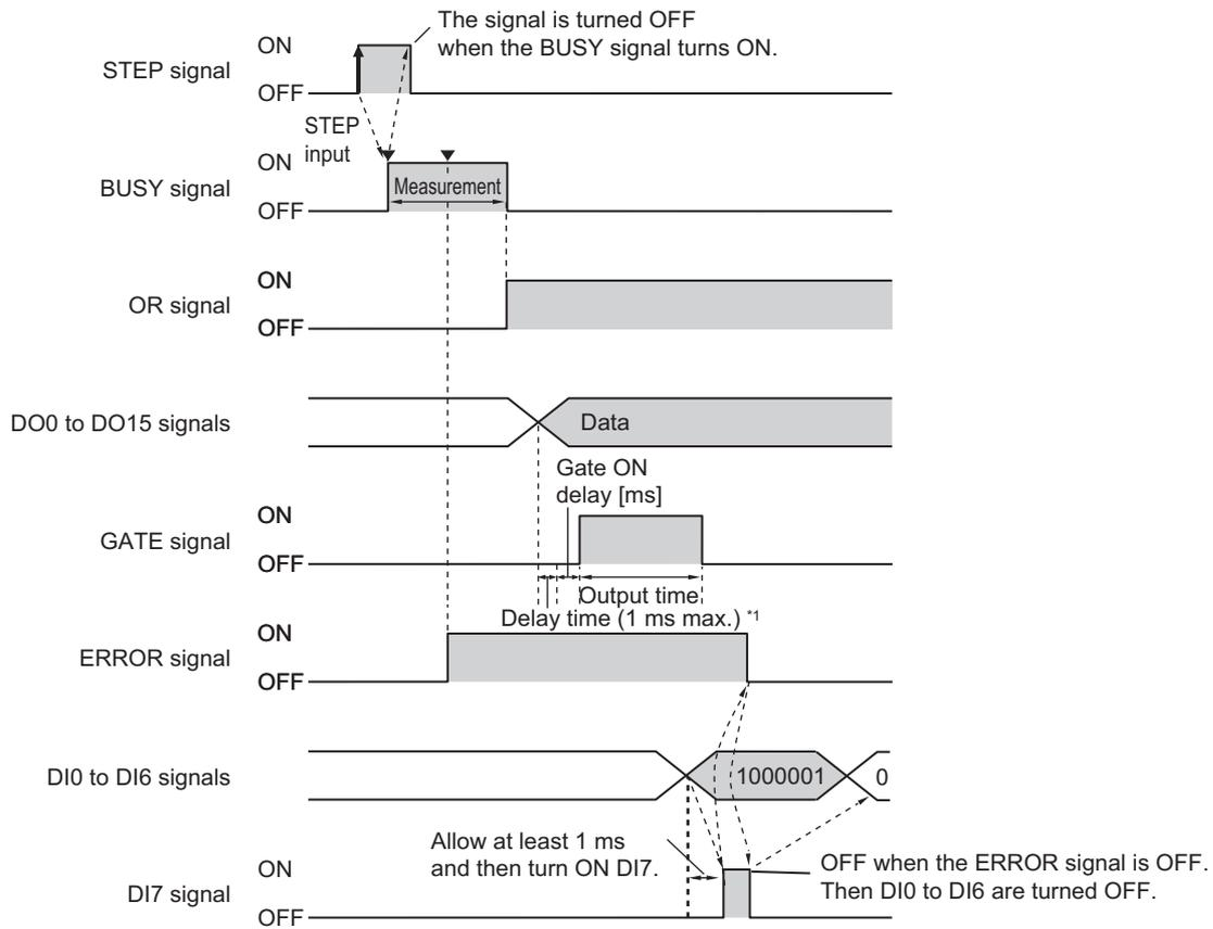
\*1 A delay of up to 1 ms will occur when the GATE signal is turned ON. (This applied only to the FH.)
