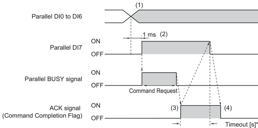
When executing continuous measurement commands, turn OFF DI7 when you want to stop continuous measurements, as shown below.
