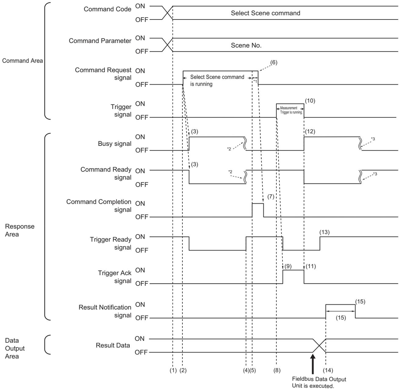
\*1: A timeout error will occur if you turn off the Command Request signal from Sensor Controller (master) within 10 seconds. Then Command Completion signal and Busy (BUSY) signal will be forced to turn off.
