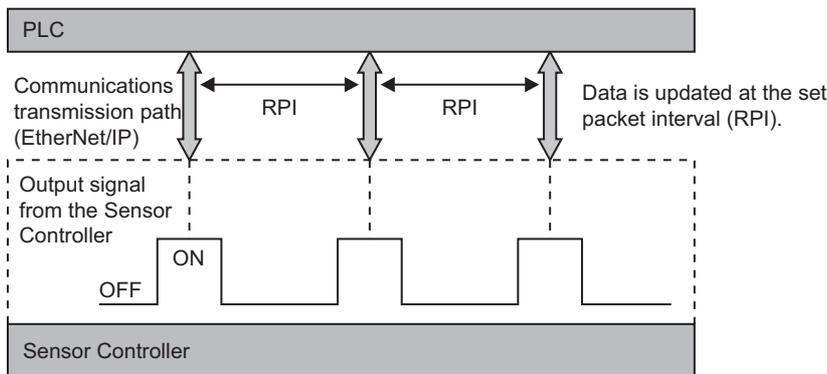
Signal changes from the Sensor Controller are affected by the RPI. In some cases the target device may not detect a change in the ON/OFF status of a signal depending on the RPI timing.
