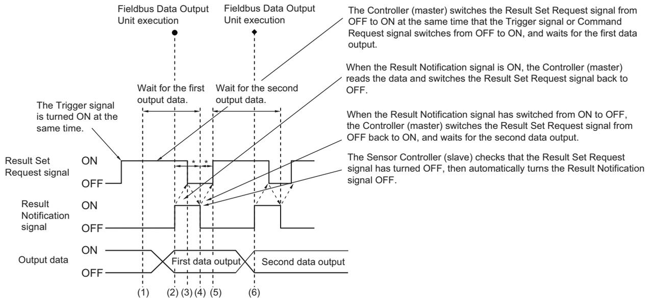
\*: A timeout error will occur if any of the following states continues for longer than the timeout time that is set in the EtherCAT settings.
