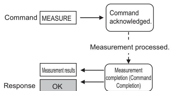
An OK response is returned when execution of the command is completed.
