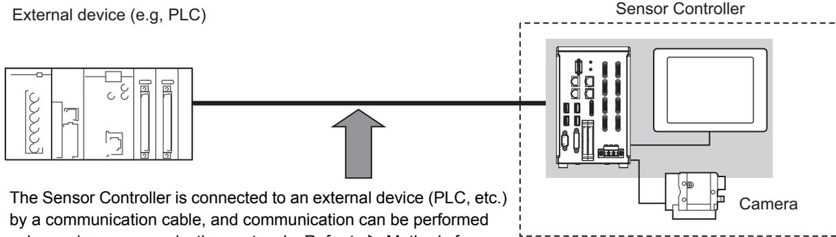
The Sensor Controller is connected to an external device (PLC, etc.) by a communication cable, and communication can be performed using various communication protocols. Refer to ► Methods for Connecting and Communicating with External Devices (p.43) for information on the different communications protocols.
