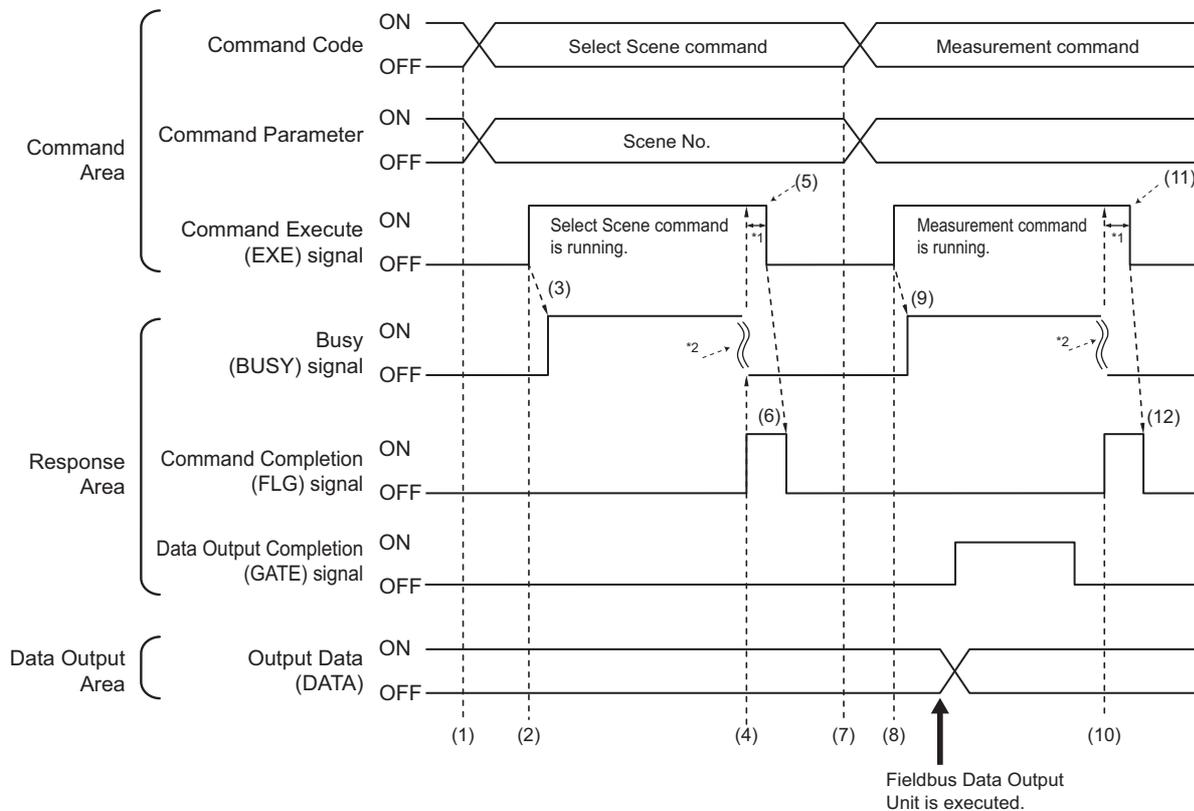
\*1: A timeout error will occur if you do not turn off the Command Execution (EXE) signal from Sensor Controller (master) within 10 seconds. Then Command Completion (FLG) signal and Busy (BUSY) signal will be forced to turn off.
