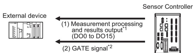
\*1: Overall judgement (OR) output is output when measurement is completed, regardless of when the Output Unit was executed.
