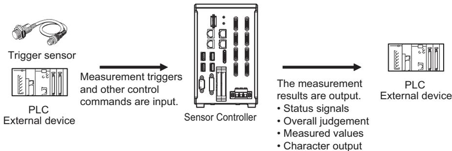
The following methods can be used to exchange data between an external device and the Sensor Controller.
