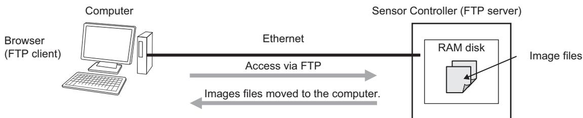
This enables you to move logged images off of the Sensor Controller's RAM disk before it becomes full.
