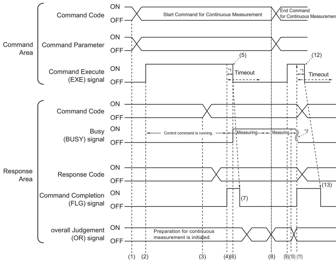
\*1: A timeout error will occur if you do not turn off the Command Execution (EXE) signal within 10 seconds after the Command Completion (FLG) signal is turned ON.
