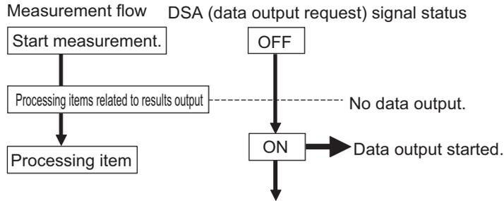
To output measurement results immediately, execute the measurement trigger and turn ON the DSA signal. The Sensor Controller does not monitor when the DSA signal changes from OFF to ON. It only checks for the ON state.
