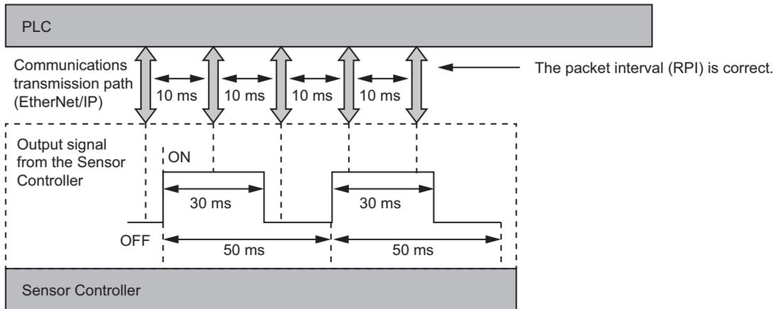
The RPI is shorter than the shortest signal time (GATE OFF: 20 ms), so the PLC can detect all output signals from the Sensor Controller.
