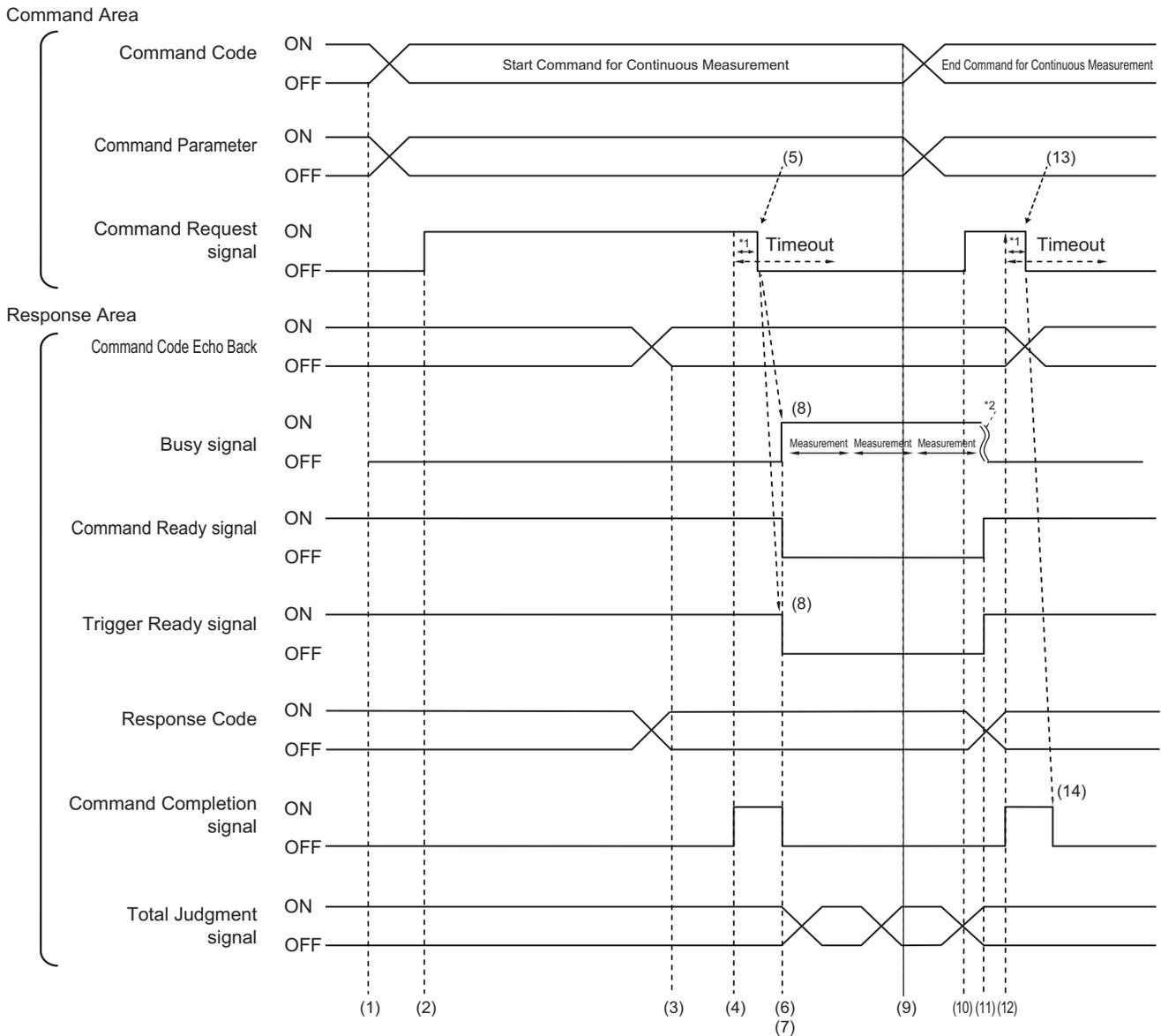
\*1: A timeout error will occur if you turn off the Command Request signal within 10 seconds after the Command Completion signal is turned ON. Command Completion signal and Busy signal will be forcefully turned OFF.
