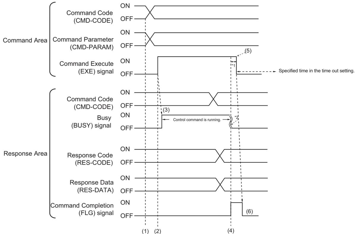
\*1: A timeout error will occur if you do not turn off the Command Execution (EXE) signal within 10 seconds after the Command Completion (FLG) signal is turned ON.
