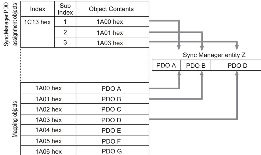
In this example, three PDOs (PDO A, PDO B, and PDO D) are assigned to index 1C13 hex (for the TxPDOs).
