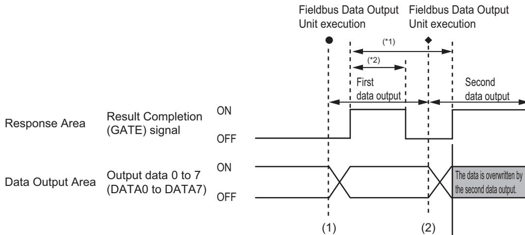
\*1, \*2: Data is output at the set output period<sup>\*1</sup> and for the set output time.<sup>\*2</sup>
