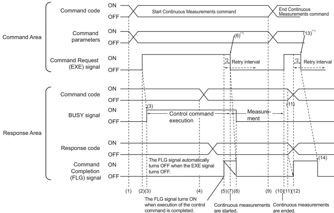
\*1: The user (PLC) turns OFF the EXE signal when the FLG signal turns ON.
