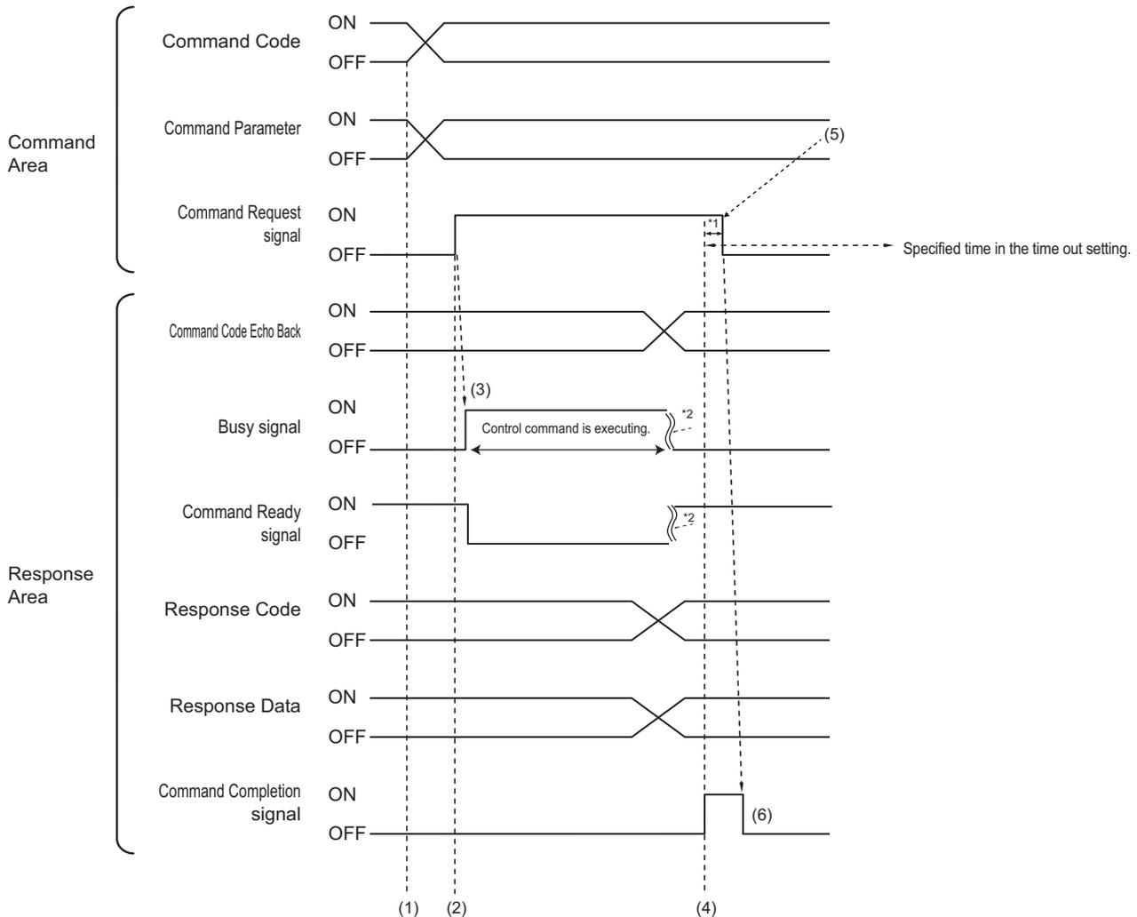
\*1: A timeout error will occur if the Command Request signals does not turn OFF within 10 seconds. Then Command Completion signal and Busy signal will be forced to turn OFF.
