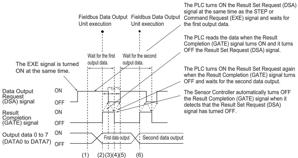
\*1 A timeout error will occur if any of the following states continues for longer than the timeout time that is set in the EtherNet/IP settings.
