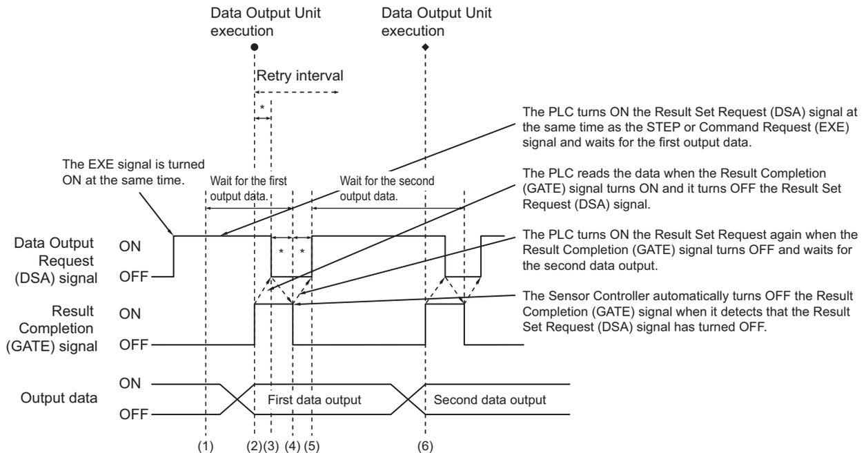
\*1: A timeout error will occur if the following states persist longer than the time set in the PLC Link settings ([Retry interval] for Ethernet PLC Link, or [Timeout] for RS-232C/422 PLC Link).
