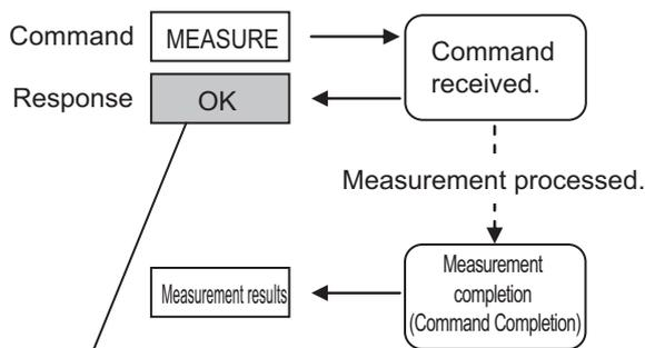
An OK response is returned when the Controller receives the command.
