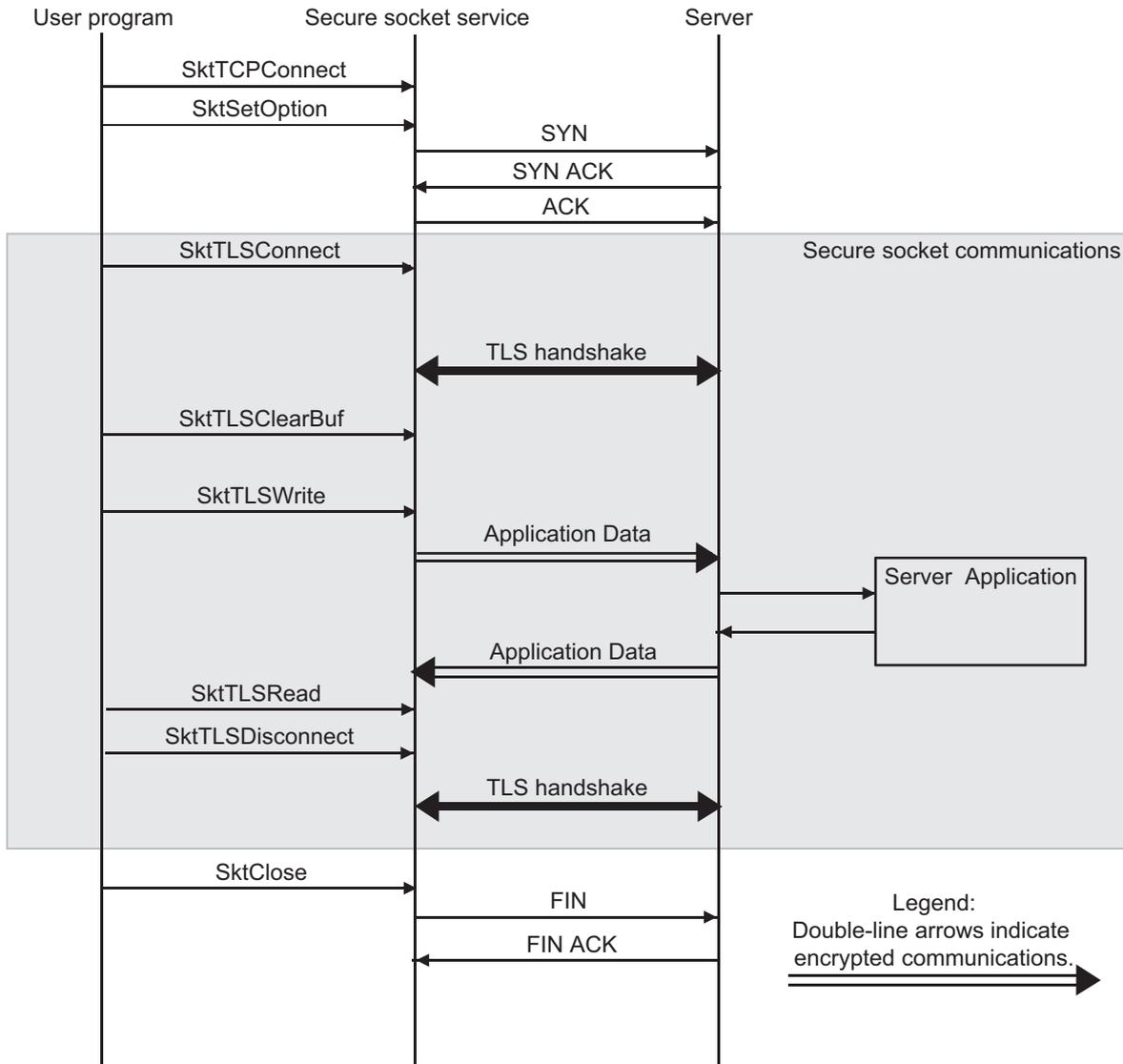
TLS Handshake exchanges and verifies the data (such as certificates) required for encrypted communications.
