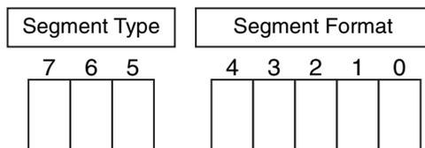
The segment type specifications are defined as follows in the CIP specifications.
