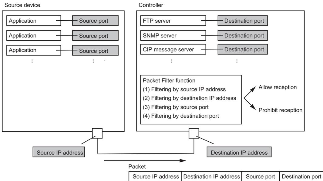
Packet Filter function can enable or disable the reception of packets using these four types of information. If the content of the packet matches the permitted content in Packet Filter settings, reception is permitted. Otherwise, reception is disabled and the packet is discarded.
