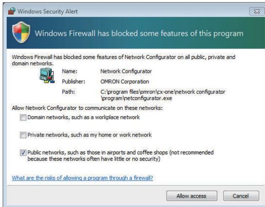
(On Windows 7) This allows USB connection and EtherNet/IP connection to the Network Configurator, and you will be able to connect to the NJ/NX-series CPU Unit via the Network Configurator.
