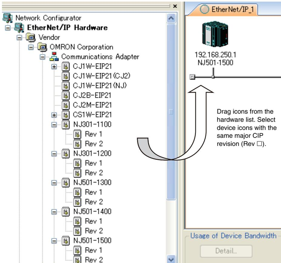
The device names and major CIP revisions (Rev □) are displayed in the hardware list. For the NJ/NX-series Controllers, device names of Units and major CIP revisions are as shown in the following table.
