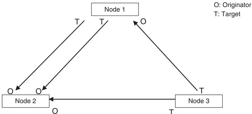
If multicast is specified for data transmission and the node sends out just one multicast packet to other nodes, it requires respective connections for them.
