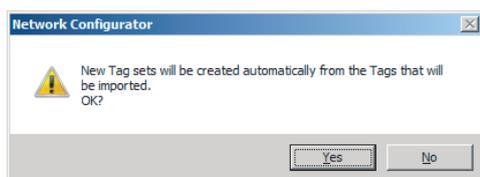
If you select the **Yes** Button in the previous step, the variables will be imported as shown below on the **Tag Sets** Tab Page. Each variable will be imported into a separate tag set and the device parameters will be automatically edited. (The variable name will be used for the tag set name.)
