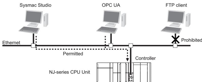
Packet Filter settings are as follows. When Sysmac Studio version 1.50 or higher is connected, it uses TCP port 443. OPC UA uses TCP port 4840.
