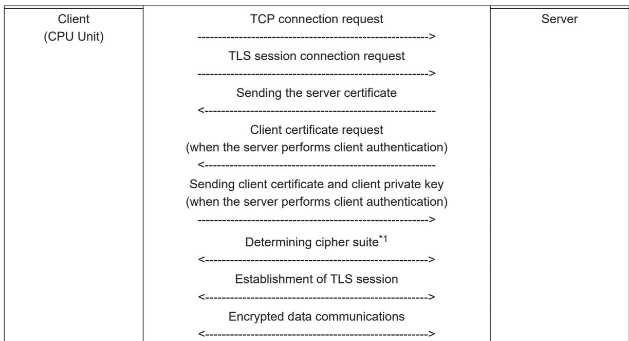
\*1. A cipher suite is a set of key exchange algorithm, key authentication method, encryption method and message authentication code.
