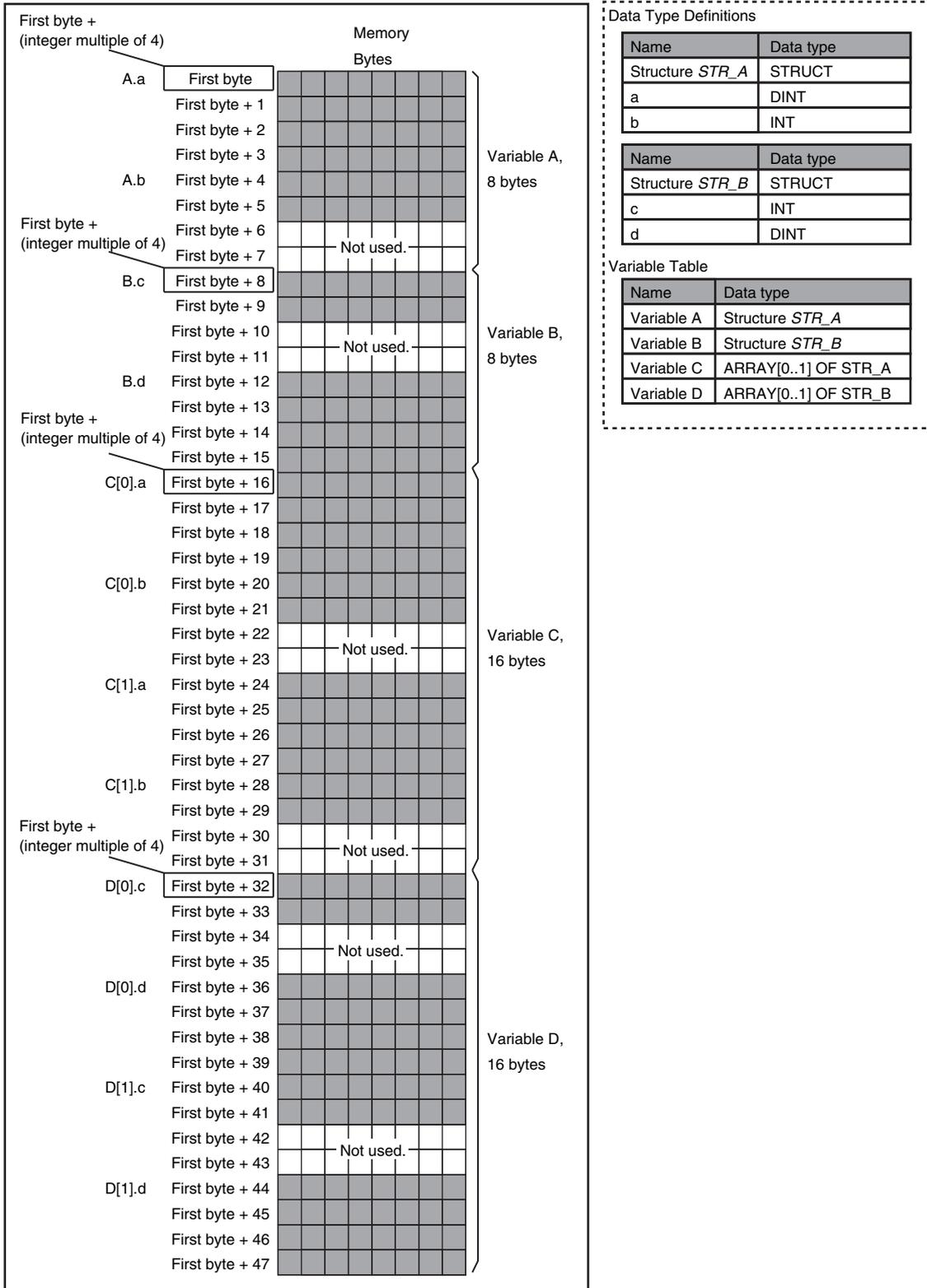
Example: The alignments and the amounts of memory that are allocated for the four variable declarations given in the following figure are given in the following table.
