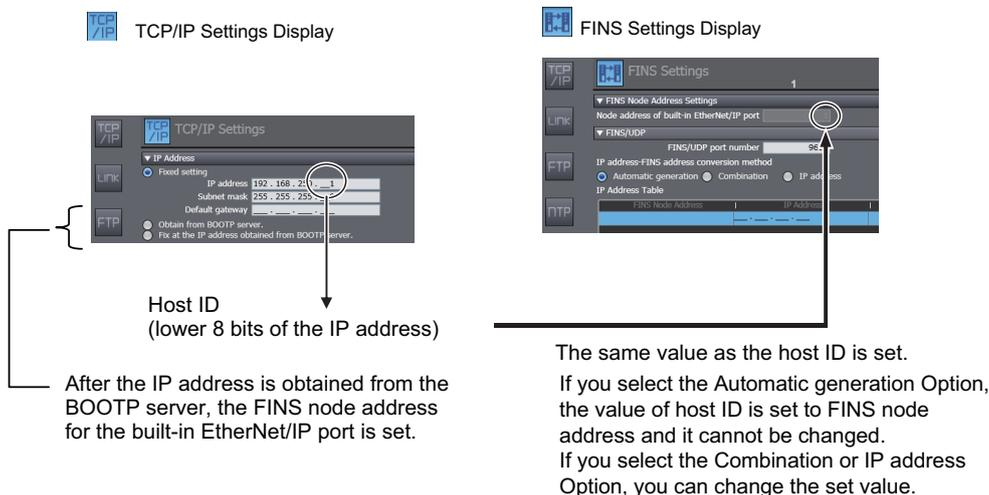
The FINS node address is required for FINS communications (e.g., to connect to the CX-Integrator and other Support Software).
