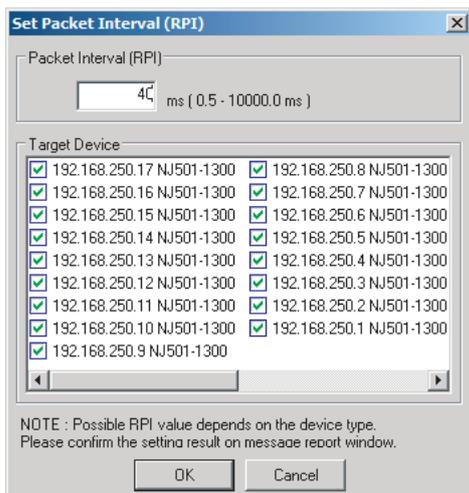
If you set the same packet interval (RPI) for all the connections, the table shows that the usage rate of allowable tag data link bandwidth is 74.50% for all the device as shown in the Usage of Capacity column, and this indicates that the shortest packet interval is 40 ms.
