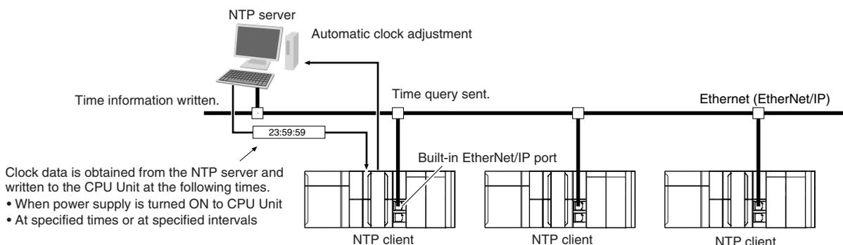
The NTP (Network Time Protocol) server is used to control the time on the LAN.
