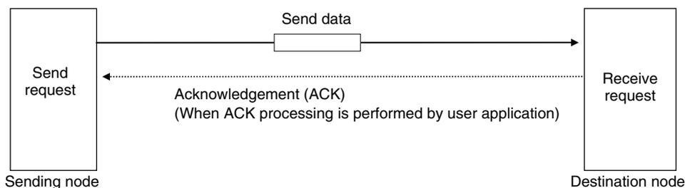
In UDP, the remote IP address and the remote UDP port number are not specified when a request is made to open a socket. The variables that store the remote IP address, the remote UDP port number, and the data to send are specified when the send request is made.
