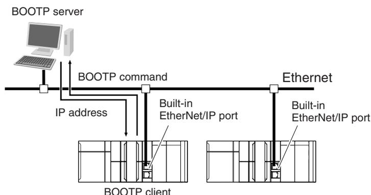
The built-in EtherNet/IP port IP address is obtained from the BOOTP server when the power is turned ON.
