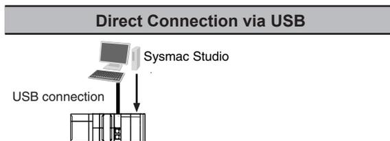
\*1. NX701 CPU Units with hardware revision A or later and NX502, NX102, and NX1P2 CPU Units do not support USB connection.
