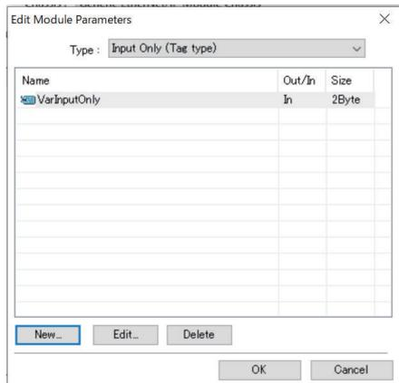
**7** Repeat steps 4 through 6 to register the required variables. Click the **OK** Button when the registration is complete.
