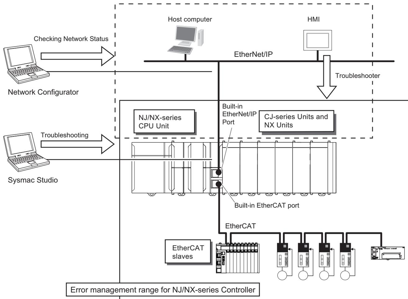
You can use the troubleshooting functions of the Sysmac Studio or the Troubleshooter on an HMI to quickly check for errors that have occurred and find corrections for them.
