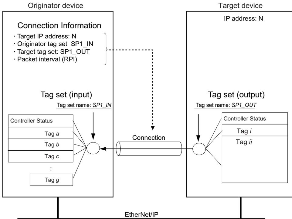
There are input (consume) and output (produce) tag sets. Each tag set can contain either input tags or output tags. The same input tag cannot be included in more than one input tag set.
