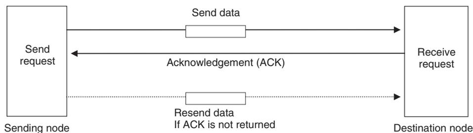
In TCP, the remote IP address and the remote TCP port number are specified when a request is made to open a socket. The variables that store the data to send are specified when the send request is made.
