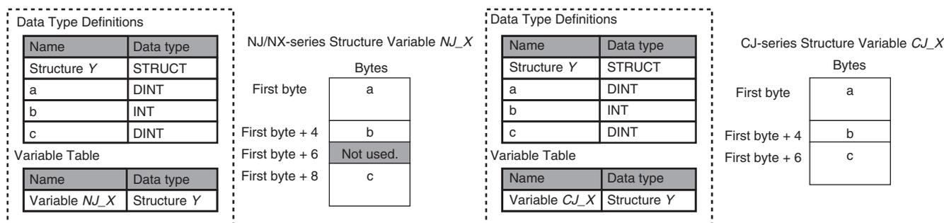
● **Method 1: Changing the Memory Configuration of the Structure Variable in the NJ/NX-series CPU Unit**
