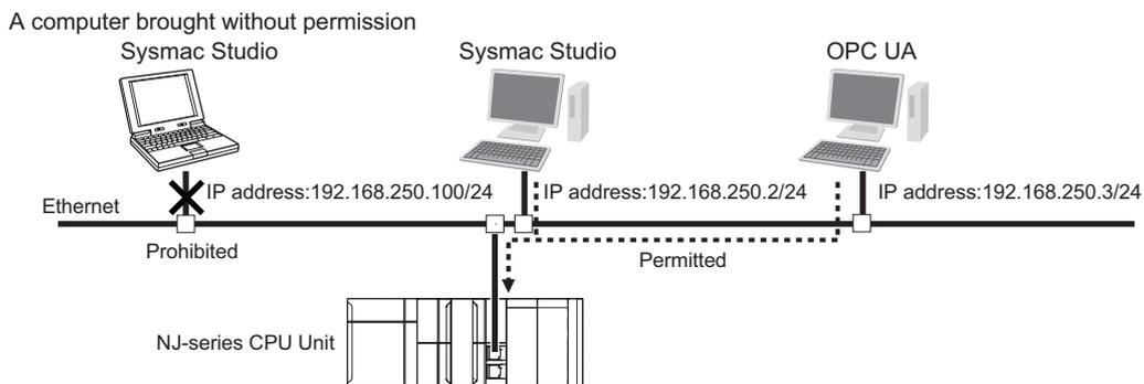
Packet Filter settings are as follows. Enter the IP address of the computer to use Sysmac Studio in the No.1 Source **IP Address** field. Enter the IP address of the computer to use OPC UA in the No.2 Source **IP Address** field.
