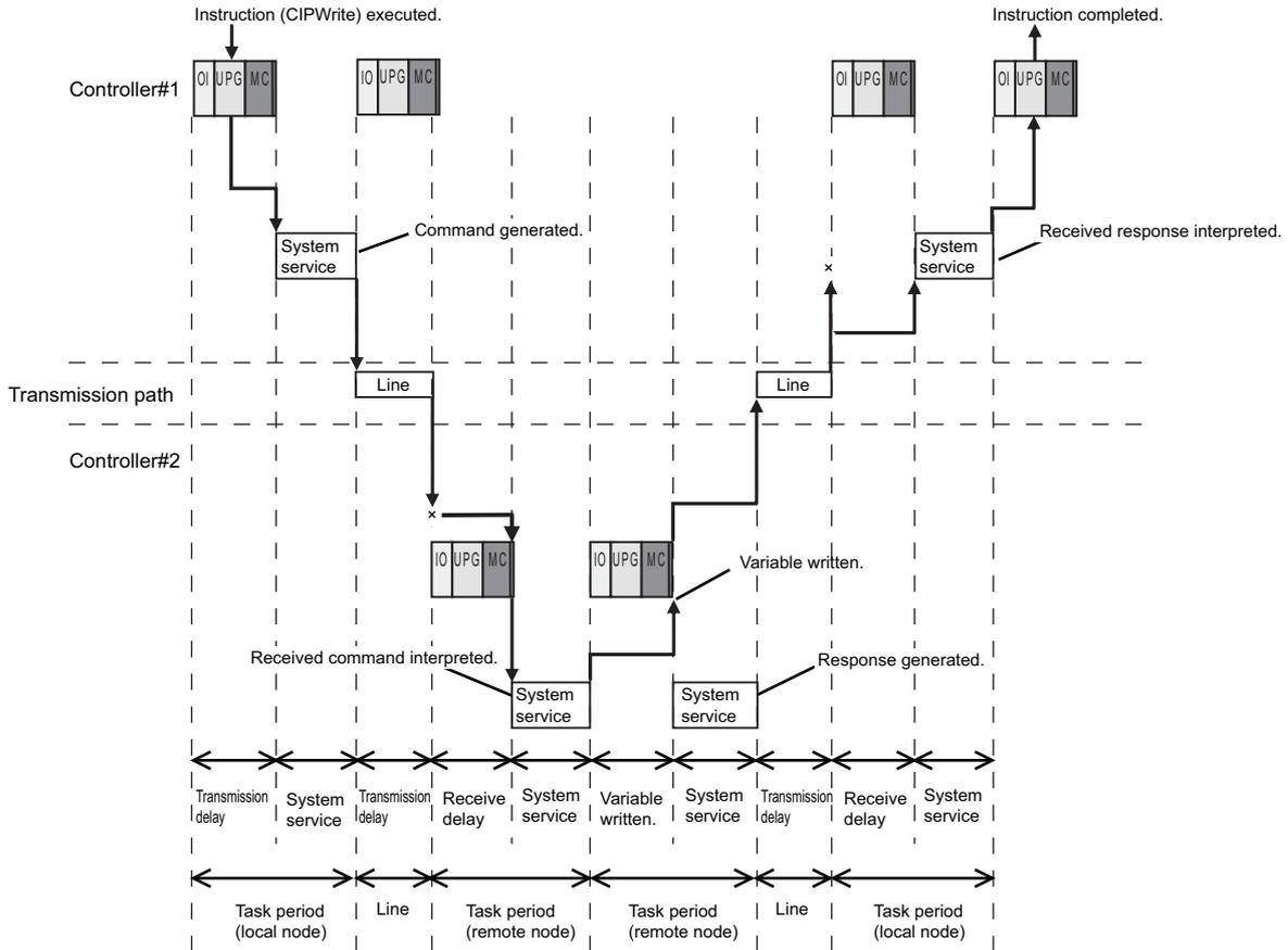
Maximum transmission delay time = Send delay + System service execution time + Transmission delay
