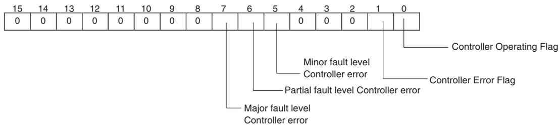
**Note** Of the flags in bits 5 to 7 that indicate the current error level, only the flag for the highest error level changes to TRUE.
