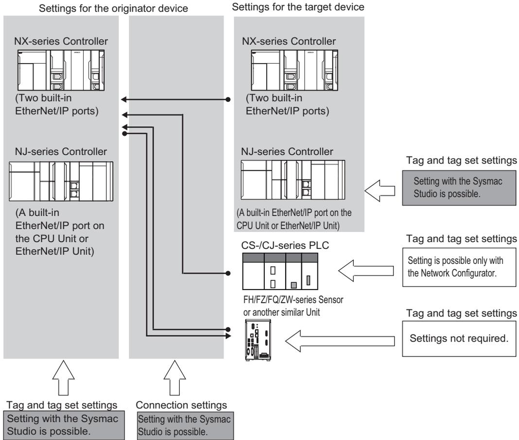
Use the Network Configurator if a CS/CJ-series PLC operates as the originator device.
