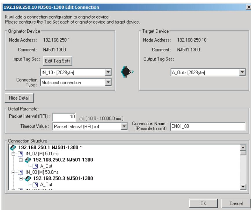
Input 10 ms as the new RPI value in the Edit Connection Dialog Box, and click the **OK** Button. The usage rate of allowable tag data link bandwidth for the device 192.168.250.1 increases to 50.17% as shown in the Usage of Capacity column, and this indicates that the RPI for the specific connection is set shorter.
