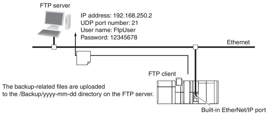
The Controller is connected to the FTP server through an EtherNet/IP network. The settings of the parameters to connect to the FTP server are given in the following table.
