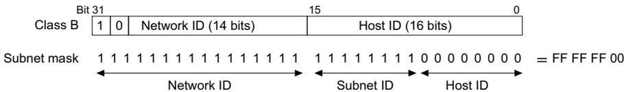
Set the same subnet mask for all of the nodes on the subnetwork. The built-in EtherNet/IP port supports CIDR (Classless Inter-Domain Routing). The subnet mask can be set to 192.0.0.0 to 255.255.255.252.
