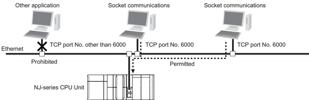
Packet Filter settings are as follows: For Protocol, **tcp** is selected and 6000 for the source port.
