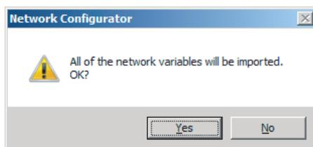
After you import the variables to the tags, click the **Yes** Button to automatically create tag sets, or click the **No** Button to set up tag sets manually.
