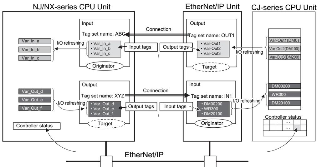
For communications between Controllers, the connection information is set in the built-in EtherNet/IP port of the Controller that receives the data (i.e., the originator).
