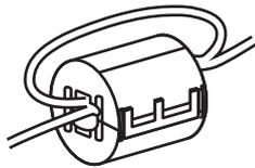
Make two loops with the cable as shown.
