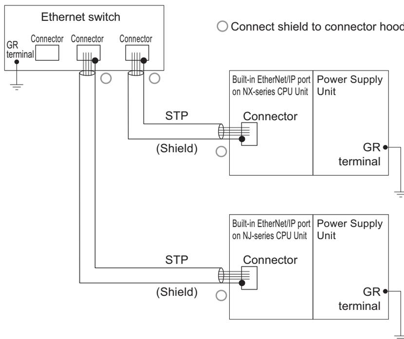
2. Connecting the shields only at the Ethernet switch side
