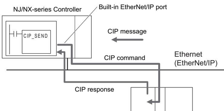
By specifying a route path, you can send CIP messages (CIP commands and responses) to a device on another CIP-based network segment via a built-in EtherNet/IP port or the EtherNet/IP Unit (CIP routing function for message communications).
