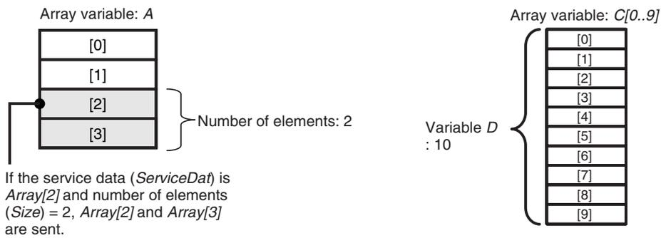
If the service data (*ServiceDat*) is *Array[2]* and number of elements (*Size*) = 2, *Array[2]* and *Array[3]* are sent.
