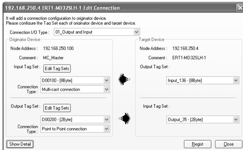
The **Connection I/O Type** list box in the upper part of the **Edit Connection** Dialog Box lists connection I/O types. Select a connection I/O type according to your application.
