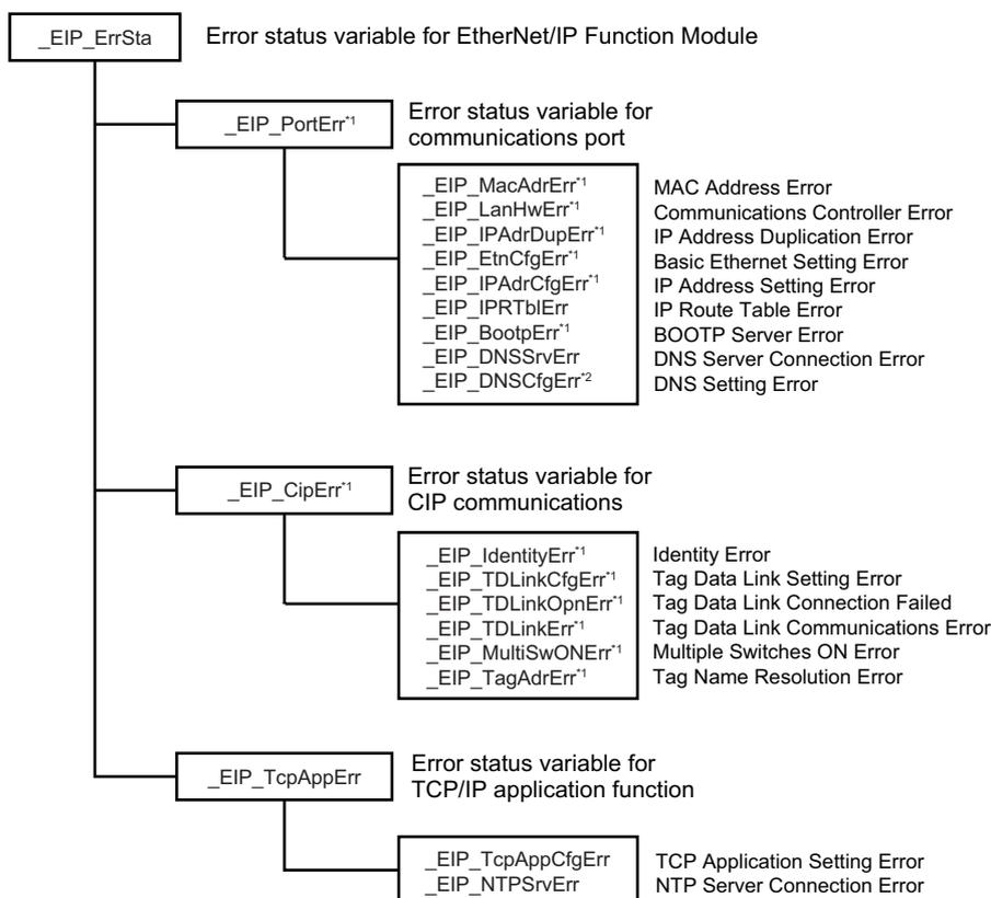
\*1. Error status variables for errors related to NX-series CPU Units are provided individually for communications port 1 and communications port 2. You can use error status variables for communications port 2 with the NX701 CPU Units, NX502 CPU Units, and NX102 CPU Units only.
