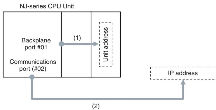
1. When Routing the Output to a Unit on the CPU Rack
