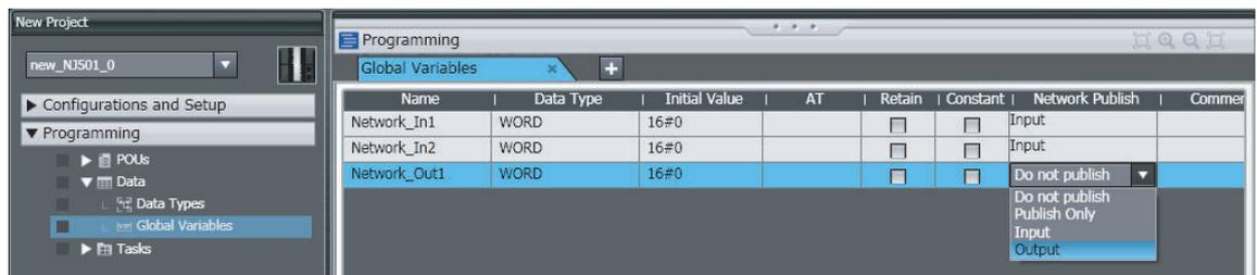
**2** Select **Export Global Variables - Network Configurator...** from the **Tools** Menu. Any global variables with **Input** or **Output** set for the Network Publish attribute are imported from the csv file through the import procedure described below (Importing to the Network Configurator).
