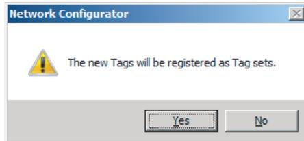
If the **No** Button is clicked, you can add more tags to the tag set. Refer to step 8 in Changing and Registering Tag Sets for details on how to register new tags first and add more tags to the tag set later.
