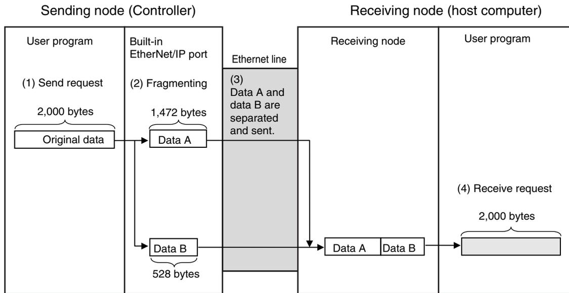
Since UDP communications are performed in datagram units as shown above, send data is restored in the original data format before it is passed to the user program.
