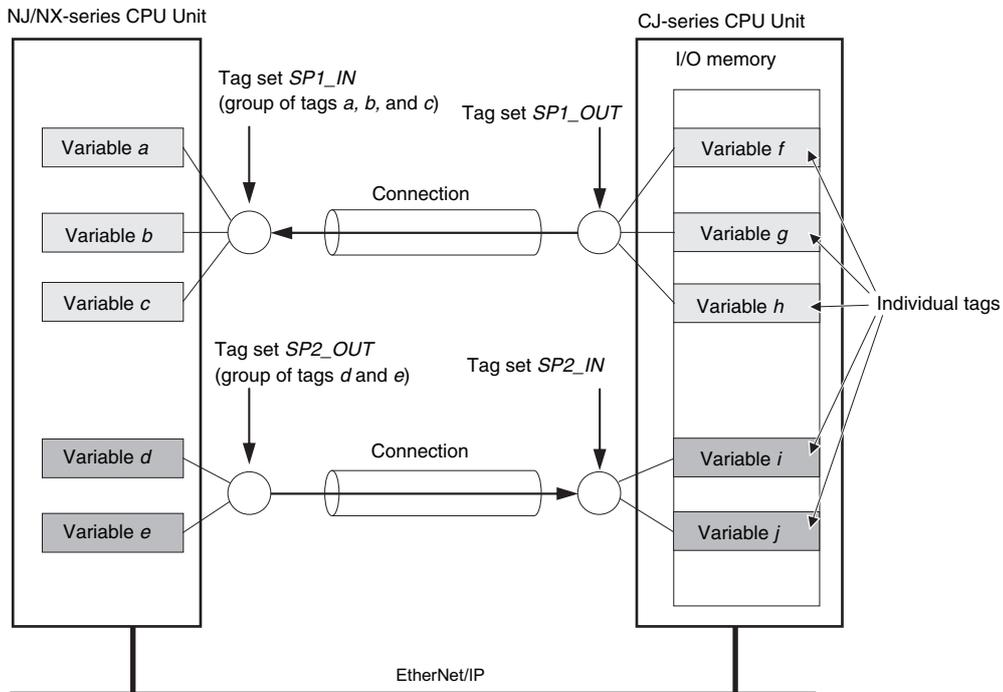
**Note** To enable a connection, each tag set must include only one of either input tags or output tags. (Both input and output tags cannot be included in one tag set.)
