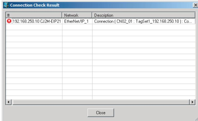
If an inconsistency is found, open the originator's **Edit Device Parameter** Dialog Box and click the **Connection** Tab. The inconsistent connection in the **Register Device List** is displayed
