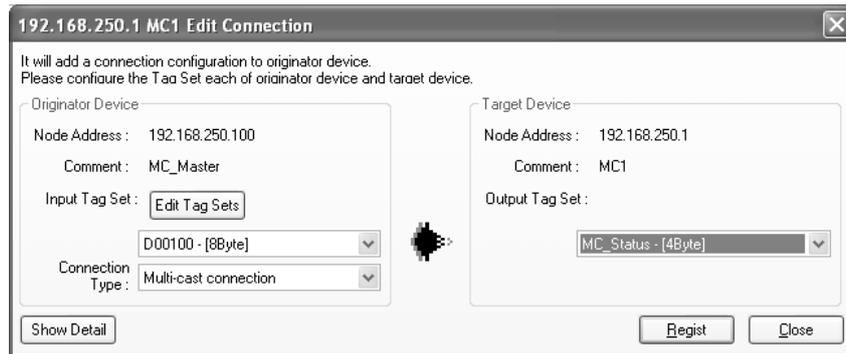
Select an output tag set from the **Target Device** Area on the right side of the **Edit Connection** Dialog Box, and then select an input tag set to receive the output tag set in the **Originator Device** Area on the left.
