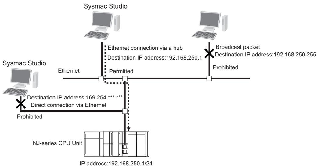
Packet Filter settings are as follows. Set the IP address for the Controller's built-in EtherNet/IP port to the destination IP address.
