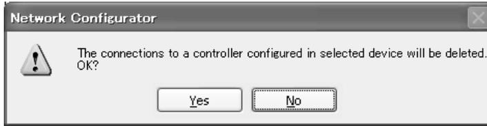
Click the **Yes** Button to delete the connections that are set with OMRON PLCs before starting the Wizard.
