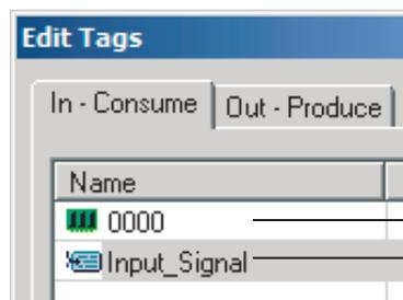
Tag that is directly assigned to an I/O memory address
