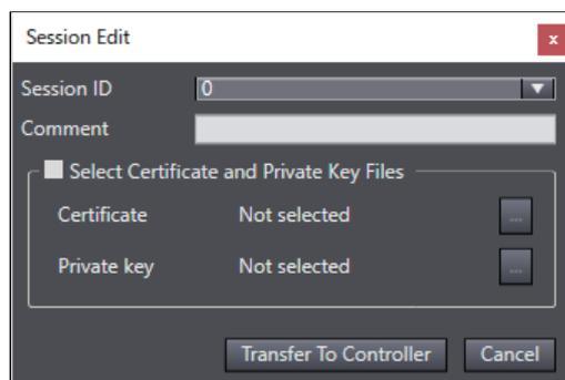
To enable secure socket communications log, select **Communications Log** to **Enabled** in the **Secure Socket Settings** Dialog Box and click the **Transfer to Controller** Button.
