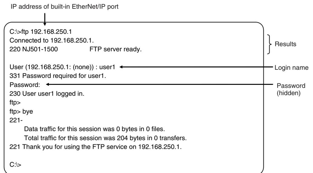
3. Enter FTP commands (underlined in the following diagram) to read and write files. The following directory tree is used in this example.
