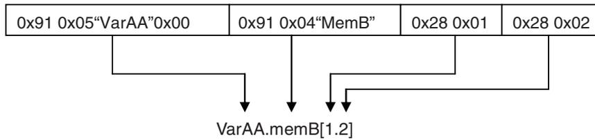
This example shows how to specify VarAA[1].MemB[1.2] for the following structure variable.
