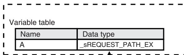
Select an extension structure for the data type of variable *A*.
