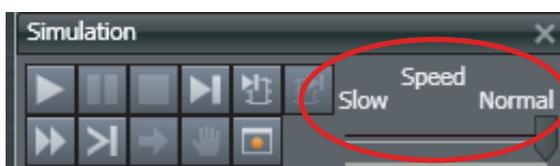
The simulation speed on the computer will change between 0.1x and 1x.
