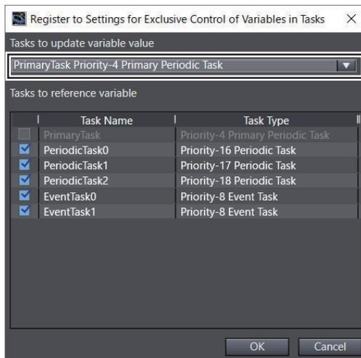
In **Tasks to update variable value**, a task to which the POU containing the specified circuit part is assigned is displayed.
