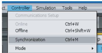
The Synchronization Window is displayed and verification of the user program and parameter settings between the Sysmac Studio and the Controller is started.
