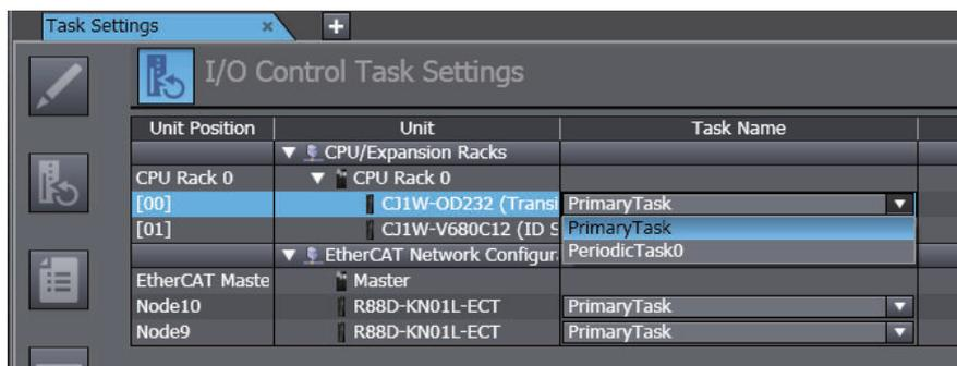
Task I/O settings can be defined only for the primary periodic task (priority 4), the priority-5 periodic task\*1, and the priority-16 periodic task\*2. You cannot define task I/O settings for priority-17 and priority-18 periodic tasks. Units specified in task I/O settings must already be registered under **Configurations and Setup – CPU/Expansion Racks** and **EtherCAT**.
