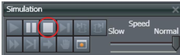
The connection to the Simulator is broken and the Simulator is exited.
