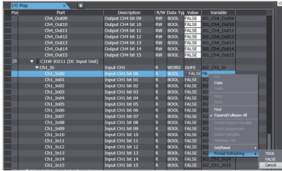
The forced value for I/O port of the selected BOOL device variable is cleared and the forced value icon disappears.
