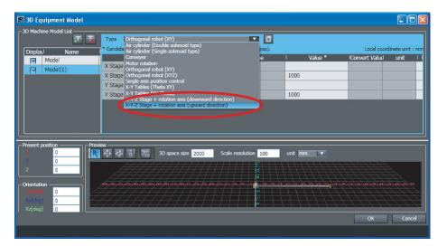
**3** Move the position of the 3D machine 500 (mm) along the X axis. Enter 500 into the "X" text box in the Present Position Area. Confirm that the 3D machine changed positions in the Preview Area.
