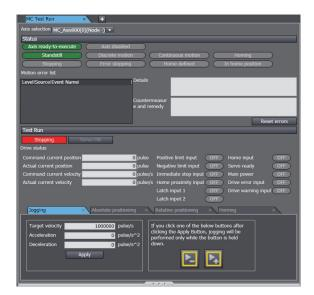
**5** Select the target axis (*MC\_Axis000*) at the upper left of the MC Test Run View.
