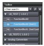
**2** Drag the library object to the ladder diagram. The function block from the library is inserted.
