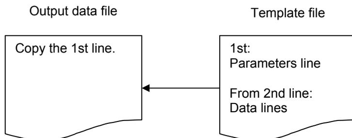
**Note** If an existing output file is specified in the Data Replay Tool, monitor data will be appended to the end of the output file. If both the output file and the output template specify "I/O memory," that of the output file is given priority.
