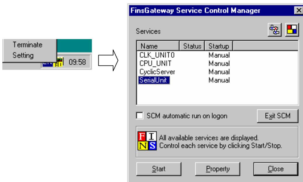
2. Select "SerialUnit" in the list of the FinsGateway Service Managers and click the [Start] button. The display will change from "List" to "Start" when "SerialUnit" starts. If the CPU Unit for FinsGateway is not started then, the CPU Unit will automatically start.
