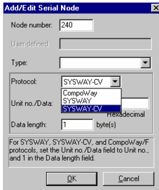
6. Select "SYSMAC WAY-CV" in the protocol of the [Add/Edit Serial Node] dialog box and click the [OK] button to return to the "SerialUnit" property.
