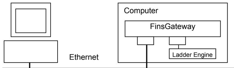
**Note** When connecting via network, the routing table must be set for FinsGateway and the relay network table for the Ladder Engine because two communications lines are required for the computer with the CX-Simulator. For instructions on setting the routing tables (including the relay network table), refer to *Section 3* of the *CX-Integrator Operation Manual (W464)*.
