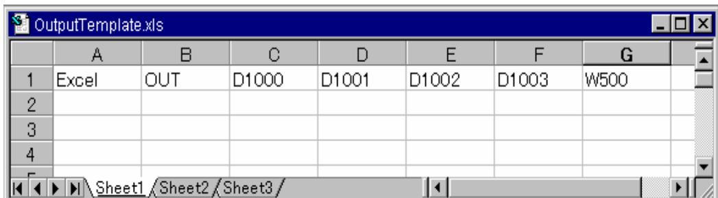
If a file output by the Data Replay Tool exists, specifying the I/O memory as an output file can be omitted by specifying the file as an output template when starting the Data Replay Tool. Specifying a template file by the Data Replay Tool will copy the I/O memory specification (parameter line) of the template file to the output file as is.
