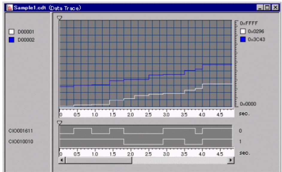
**Note** Refer to the *Data Trace/Time Chart Monitoring* of *CHAPTER 4 - Reference of PART 1: CX-Programmer* in the *CX-Programmer Operation Manual (W446)* for how to operate the data trace and time chart monitoring.
