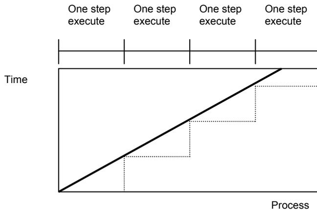
Note: The dashed line shows the time elapse in the virtual cycle time.
