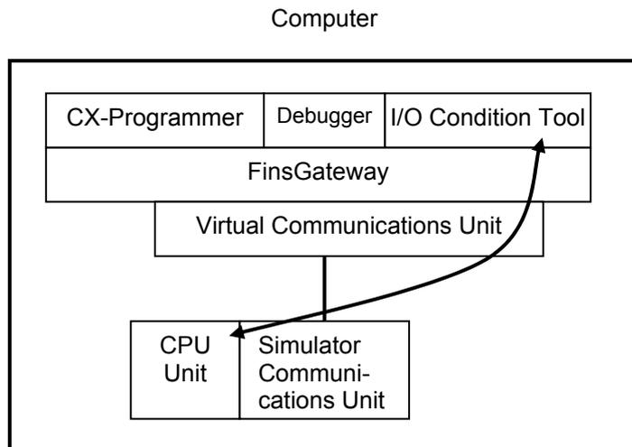
The I/O Condition Tool operates independently of the Debugger.
