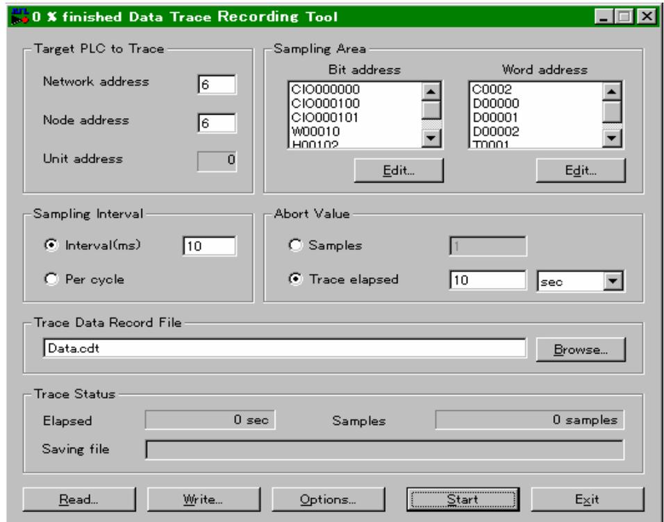
2. Confirm the FINS address (network/node address) for the target PLC is correctly set.
