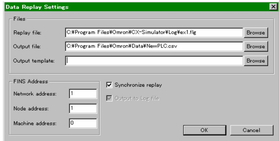
2. Specify the Data Replay File. The [Browse] button can be used, too. The Command log file (.flg), Data Trace File (.cdt), and Data Replay File(.csv) can be specified.
