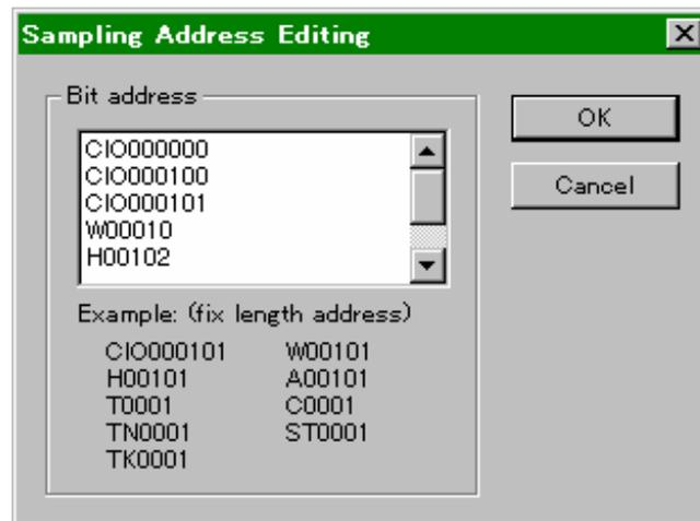
4. Click the list of [Bit address] and key-in the address of the I/O memory area to be saved.
