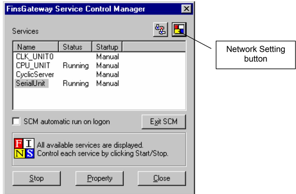
3. Click the [Network Setting] button to display the [FinsGateway Network Navigator] window.
