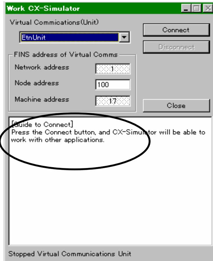
5. Set the FINS address displayed in the [Guide to Connect] to the target FINS address of the application program.
