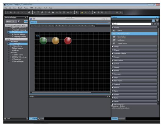
8 Match the size of the Momentary Button object with the size of the Bit Lamp object.
