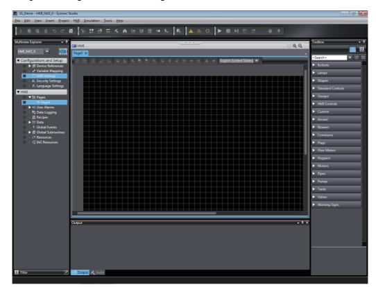
**2** Overlay a Momentary Button object on a Bit Lamp object to implement the actual button. Click *Lamps* in the Toolbox and then drag a Bit Lamp object to the page.
