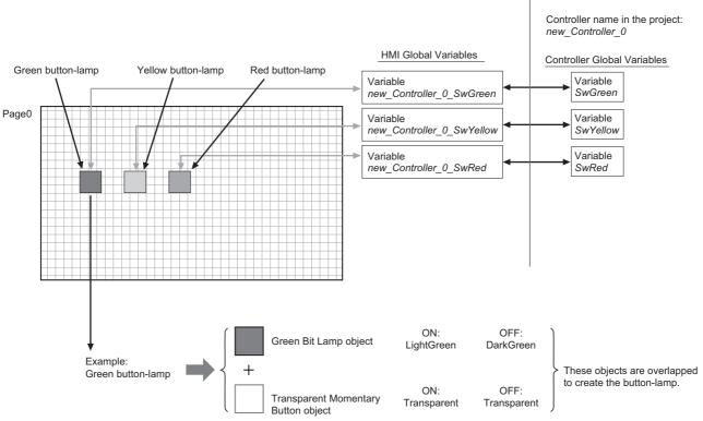
Position the Bit Lamp objects and set the colors as shown below for the TRUE and FALSE status in the Controller.
