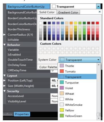
**11** Assign a variable to the Momentary Button object. Set **Behavior** – **Variable** in the properties to new\_Controller\_0\_SwGreen.
