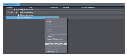
The Controller global variables are automatically mapped to the HMI global variables.
