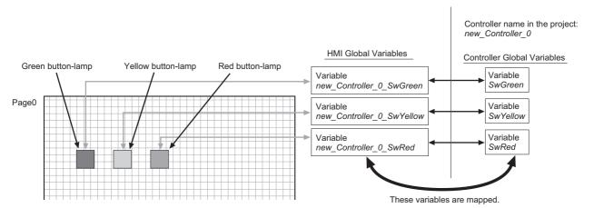
Double-click Variable Mapping under Configurations and Setup in the Multiview Explorer. Or right-click Variable Mapping under Configurations and Setup in the Multiview Explorer and select Edit from the menu.
