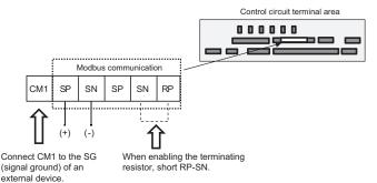
SP and SN terminals with the same names are internally connected respectively, so they can be used for wiring multiple terminals.
