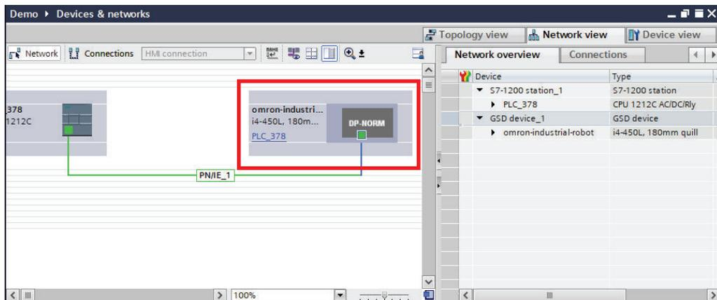
**5** Assign the IP address of the robot with TIA Portal.
