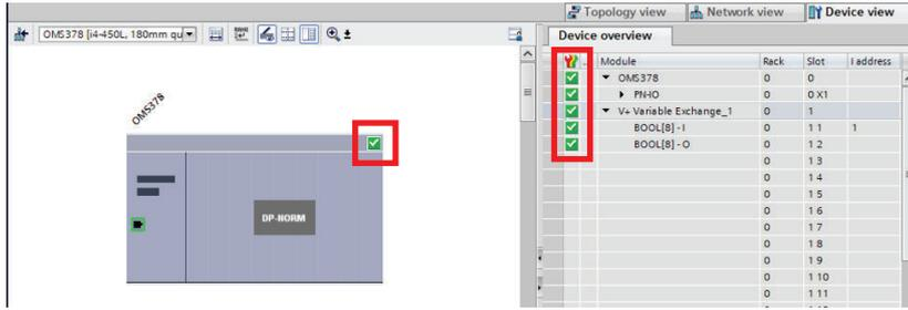
**18** Confirm data exchange by checking the following areas in the ACE software.
