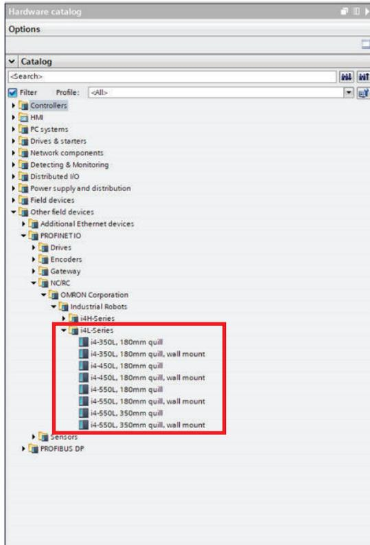
**4** Add the robot device to the Network view with TIA Portal.
