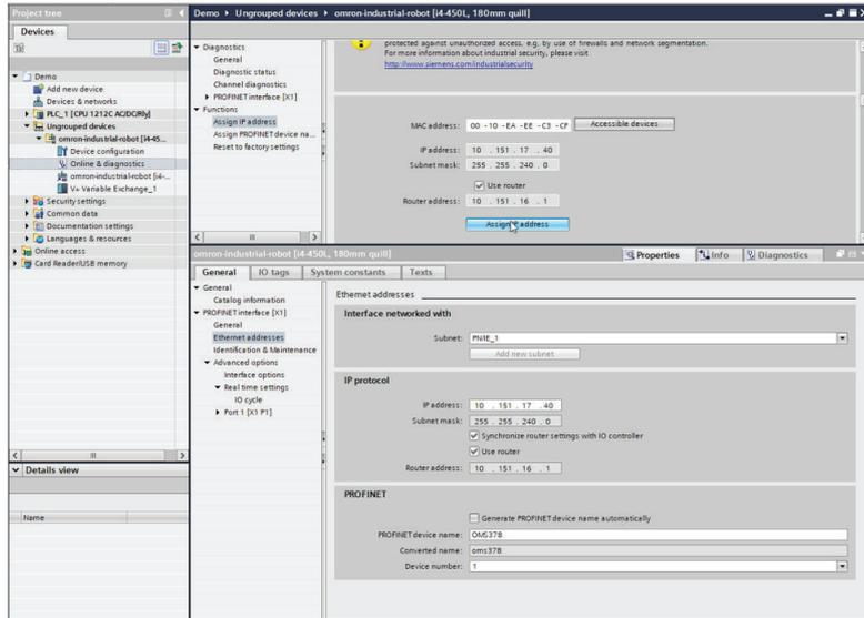
**6** Assign a unique device name to the robot in TIA Portal.
