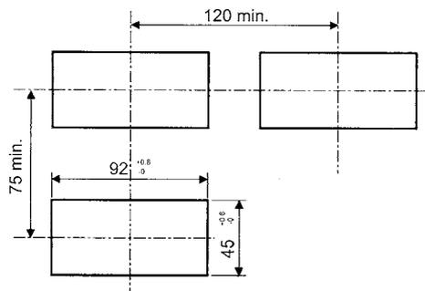
Fit the product into a rectangular panel cutout, put the adapter in the fixing grooves on the left and right surfaces of the rear case, and push the product until the gap between the product and the panel surface is minimized.
