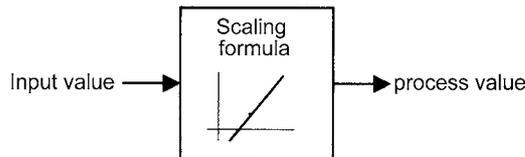
Scaling allows conversion of input values to process values in easy-to-understand notation.
