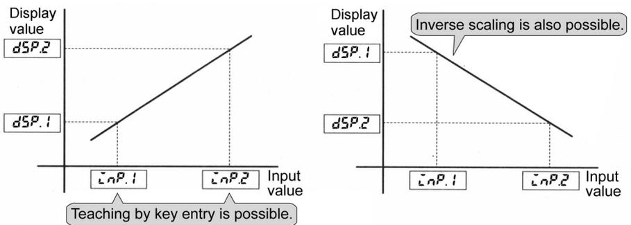
Inverse scaling where readout decreases with increasing input is also possible.
