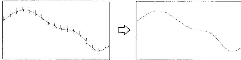
The average processing of the K3MA provides a simple average (an arithmetic mean).
