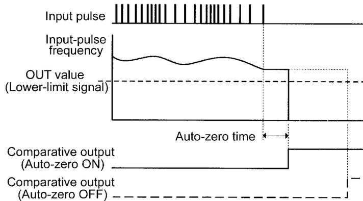
To eliminate such a situation, K3MA-F has an **auto-zero** function that shifts the input pulse frequency to zero forcedly when no pulse is received for a predetermined time.
