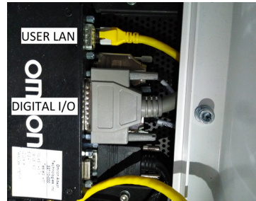
USER LAN and DIGITAL IO connectors (LD Platform Core front, upper)
