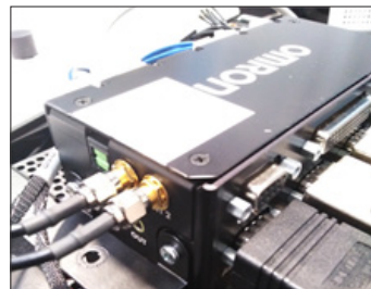
WiFi antennas connection Right side of the Core
