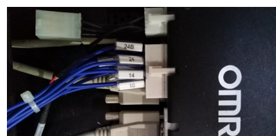
USER INTERFACE connector (LD Platform Core rear, upper)
