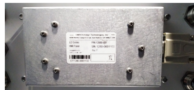
Omron Operator panel
