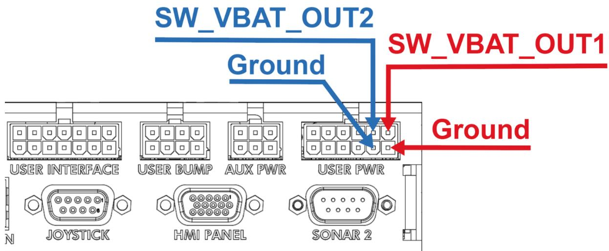
Below is the interface circuit. It consists of the battery's unregulated voltage, which is within the range of 21 V to 30.3 V (derived from the USER PWR port on the Core). The circuit elements shown below are there for protective reasons.
