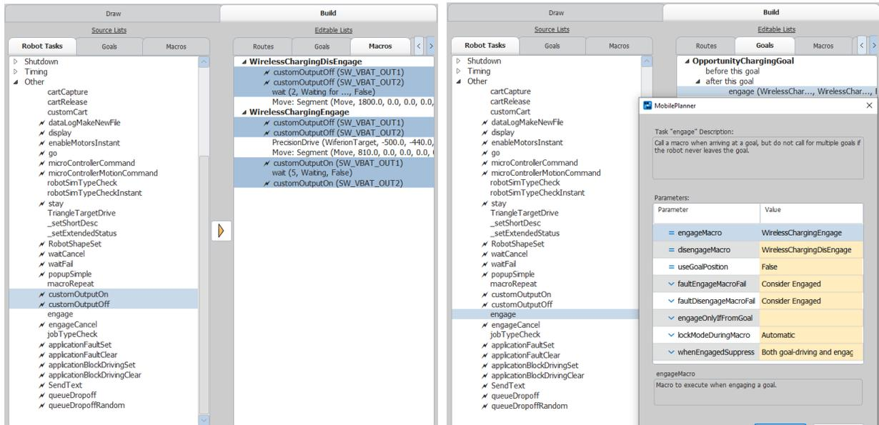
To start charging reliably for opportunity charging, the timing of the I/Os needs to be controlled in a certain way (as explained in the previous section). To achieve this reliability, it is required to trigger the I/Os in the sequence shown in the previous figure. These are some key points to note:
