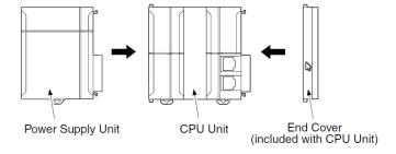
After joining the connectors between the Units, use the sliders at the top and bottom of each Unit to lock the Units together. Lock the sliders firmly into place.
