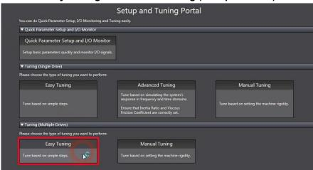
Select **Mechanically Linked Axes** as the target application, select the drives to tune, and click the **OK** Button. The gantry system has an axis configuration with mechanically linked axes.
