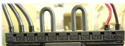
Example: CNA for 100V/200V (up to 1kW)
