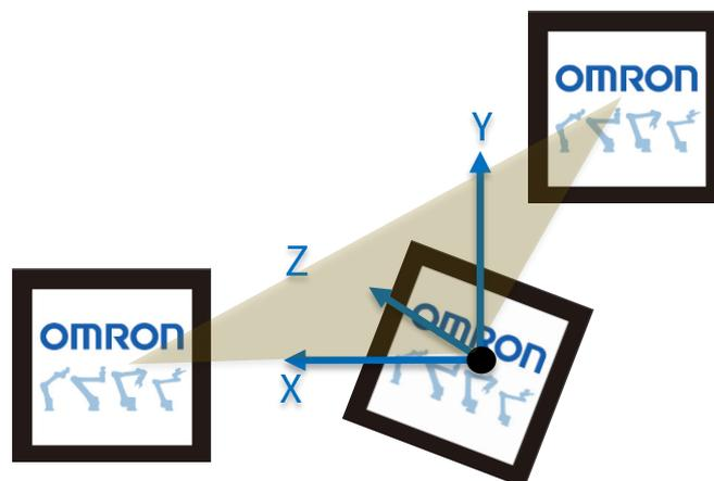
Figure 2: Vision base created on the basis of three OMRON Landmarks
