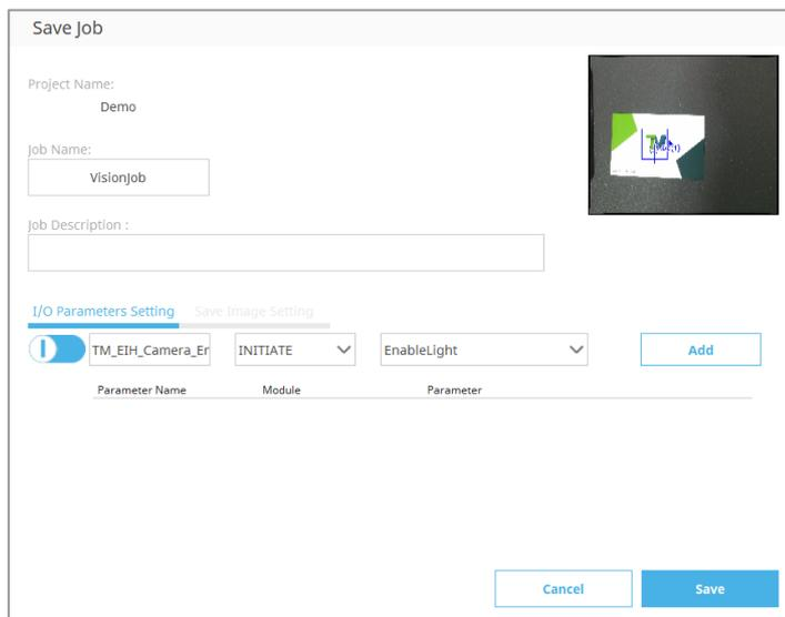
Figure 7: Set I/O Parameters Based on Results
