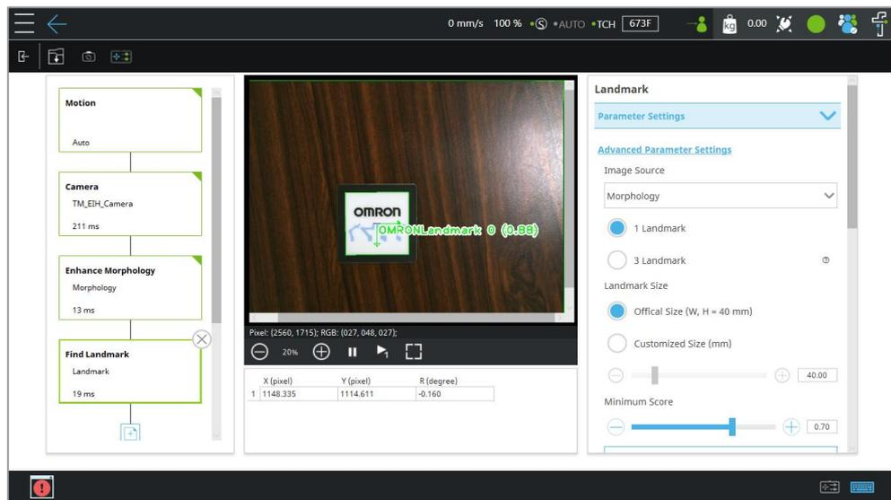
Figure 11: Landmark Positioning (1/2)
