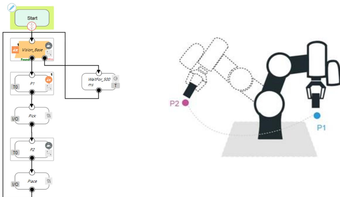
Figure 6: The Flow of Pick and Place
