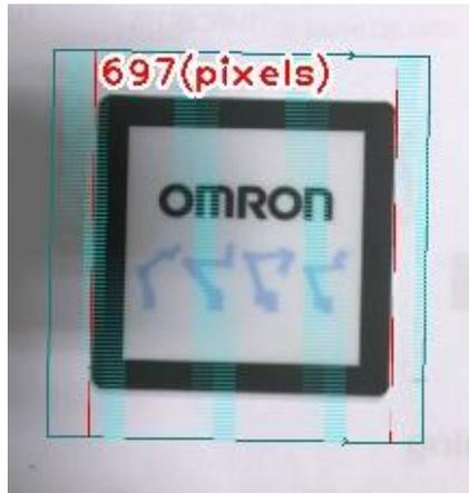
Figure 36: Caliper (Peak-to-Peak Width) Example
