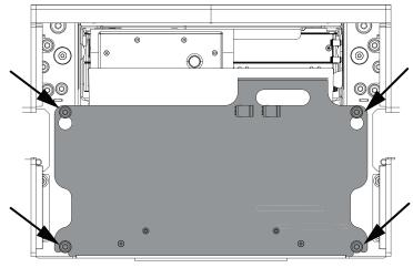
**5** Slide up the battery compartment cover and remove it from the AMR.
