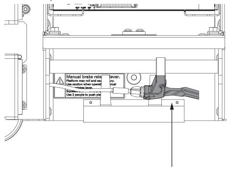
Ensure brake lever returns to original position after releasing.
