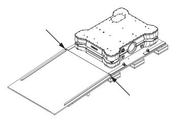
15 Place the large chock removed in the previous step at the base of the ramp. This provides a smooth transition from the ramp to the floor.
