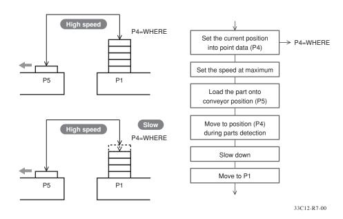
4. Use a STOPON condition in the MOVE statement for sensor detection during movement.
