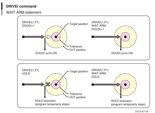
The WAIT ARM statement are used to execute the next command after the axis enters the tolerance range.
