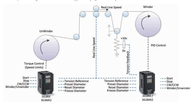
Note: In this specific Winder/Unwinder Application program, the line speed is given through the analog input O2 (RX)/OI (MX2) and the tension feedback through analog input O.
