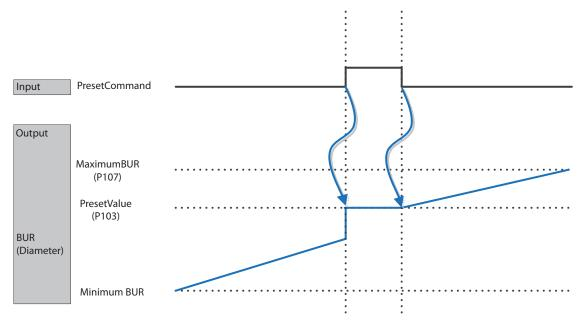
BUR = Build Up Ratio (Diameter Ratio)
