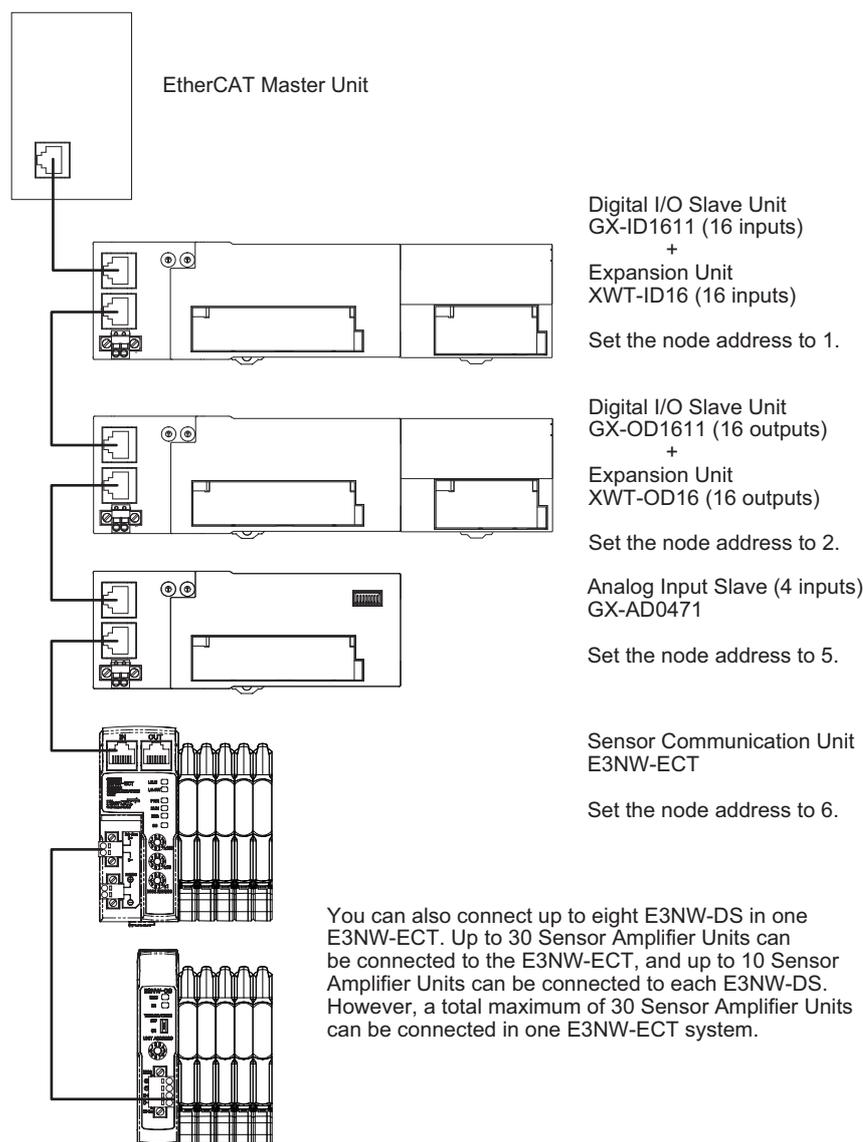
Although it is not shown in the figure above, supply the unit power and the I/O power separately.
