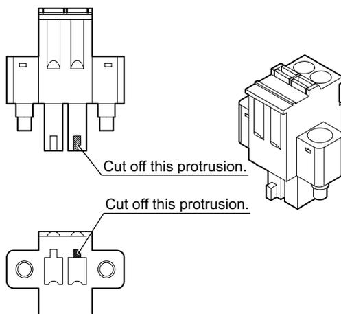
● **E3NW-DS Sensor Distributed Sensor Units**
