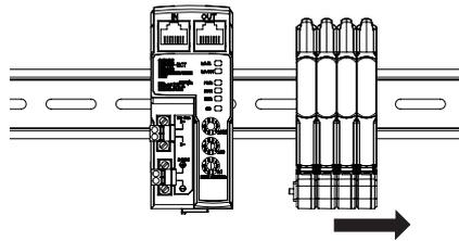
2. Keep the Sensor Communication Unit pressed against the DIN Track as you lift it up, and then off.
