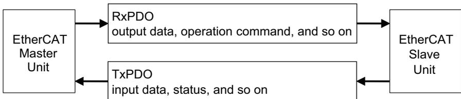
It is possible to hold multiple objects in the EtherCAT application layer so that various process data of EtherCAT Sensor Communication Units can be transferred. The details of process data are described in PDO Mapping Objects and Sync Manager PDO Assignment Objects. E3NW-ECT EtherCAT Sensor Communication Units support PDO mapping for I/O control.
