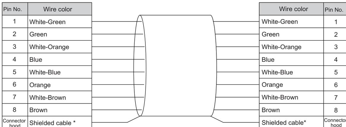
\* Connect both ends of cable shielded wires to the connector hoods.
