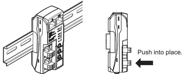
3. Remove the protective cap from the right side of the Sensor Communication Unit. Then, slide the Sensor Amplifier Units against the Sensor Communication Unit with the tabs aligned with the notches in the connector area. Press them together until they click into place.
