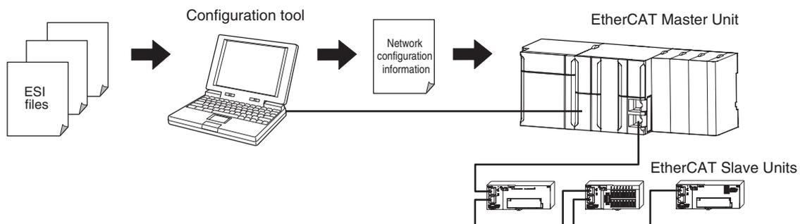
Communications are started according to the communications settings and the network configuration in the ESI files that are installed.
