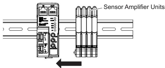
4. Use the DIN Track End Plates (PFP-M) that are provided to remove any gaps between the Units and secure them in place. Replace the protective cap that you removed in step 3 to the Sensor Amplifier on the right end.
