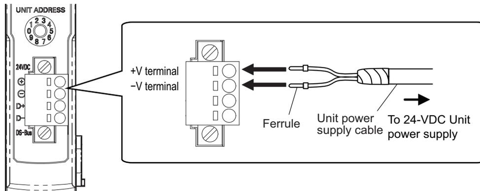
Attach ferrules to the Unit power supply cable wires and connect them securely so that they do not come loose.
