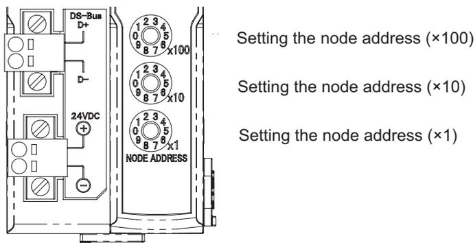
Note that the node address set values vary as shown below when the EtherCAT Master Unit is made by OMRON or by other manufacturers.
