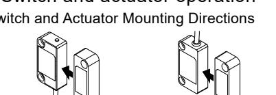
**Switch and Actuator Operating Directions**
